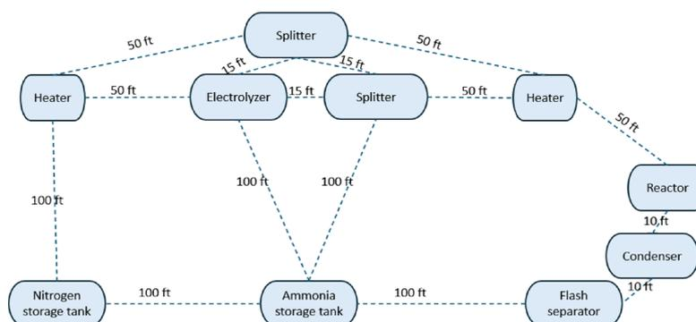
Figure 8 Equipment spacing of green ammonia plant.
