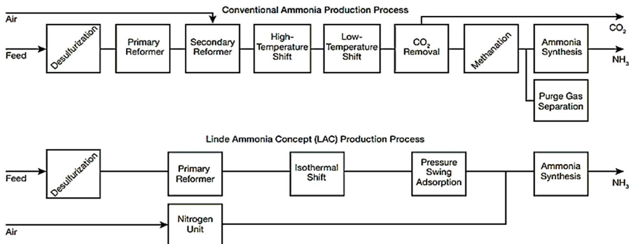
Figure 2 A block flow diagram of the Haber-Bosch process [6].
