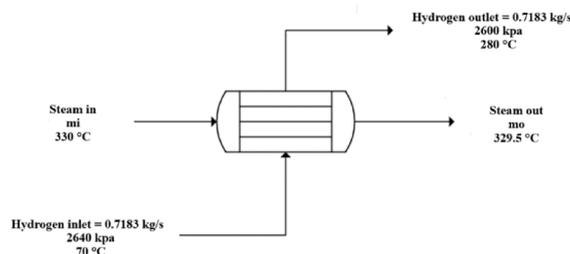
Figure 7 illustrates the heat exchanger inlet and outlet streams.
