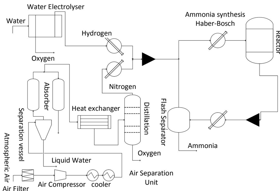
Figure 5 Illustrate the flow diagram of the green ammonia synthesis process.
