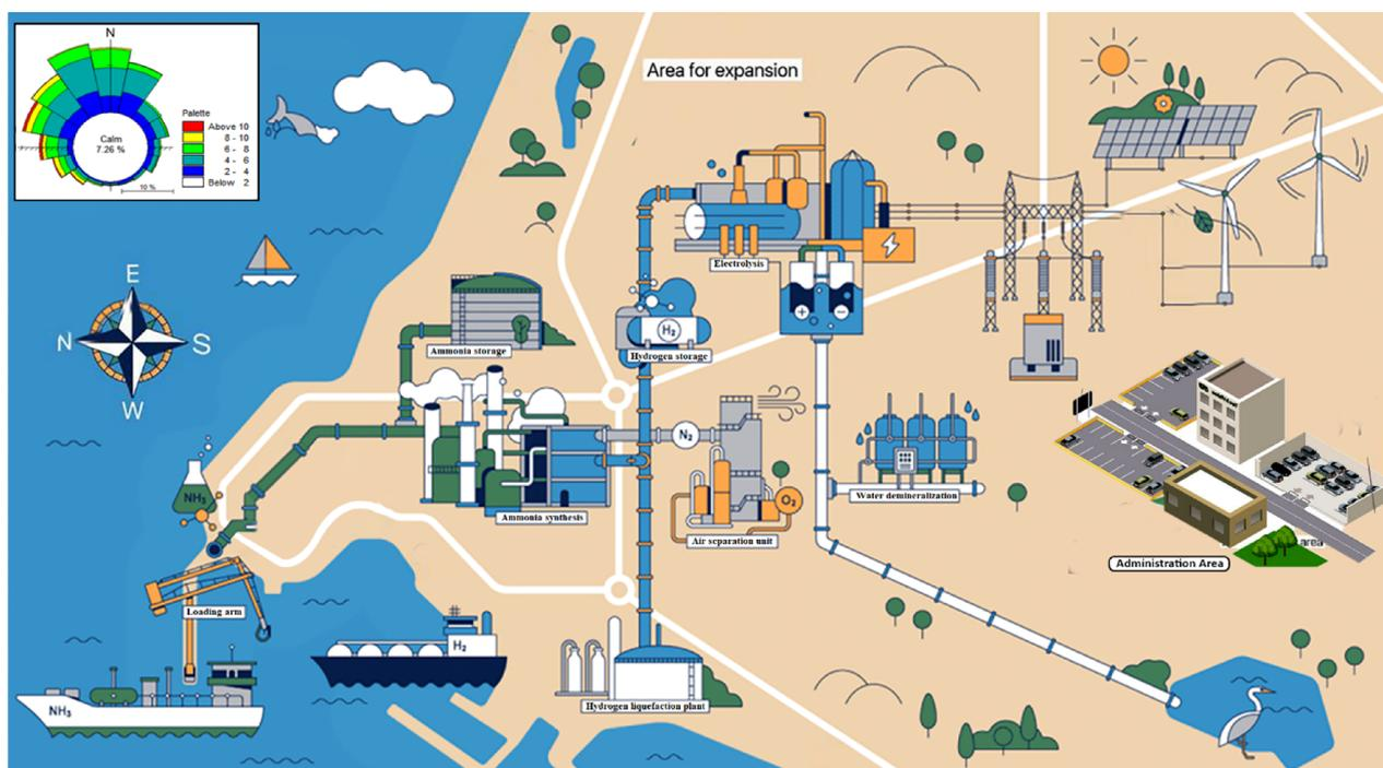
Figure 10 Plant layout for Green Ammonia production at Damietta Port.
