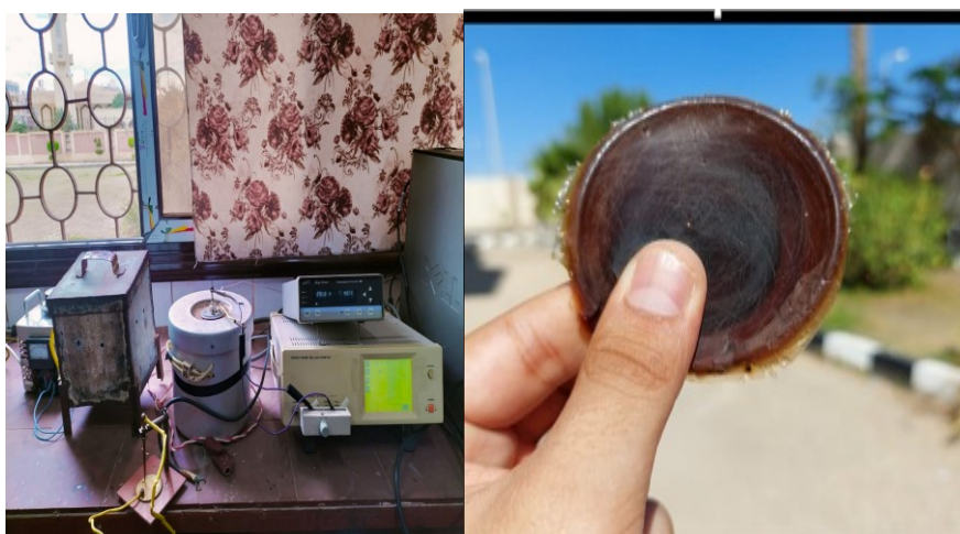
Figure 1. A HIOKI 353250 LCR Hi tester on a frequency range of 0.1 Hz to 5 MHz with a 0.1V applied voltage.
