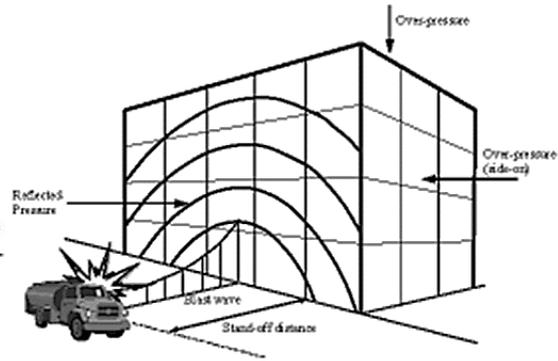
Figure 3: Blast loads on a building
