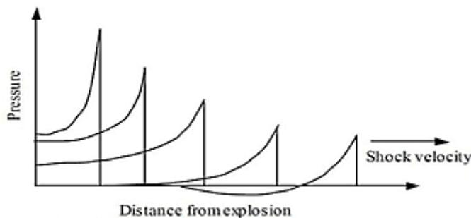
Figure 1: Blast wave propagation
