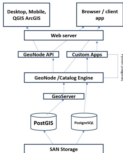
**Figure (3)** shows schematic diagram of the geoportal components and requirements.
