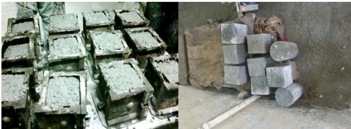
**Fig. 5b.** Compaction on concrete cubes and curing
