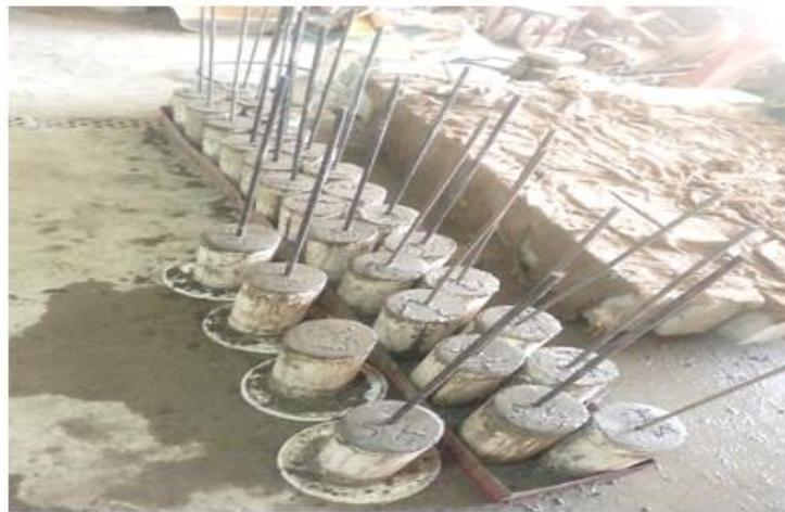
**Fig. 5a.** Compaction on concrete cubes and curing
