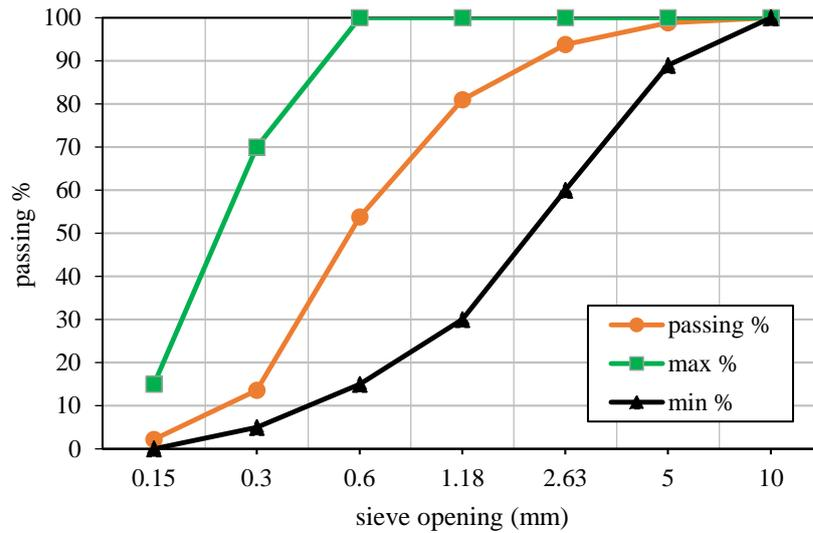
**Fig. 1. Grading curve of sand**
