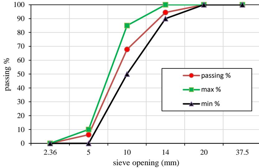
Fig. 2. Grading curve for crushed dolomite
