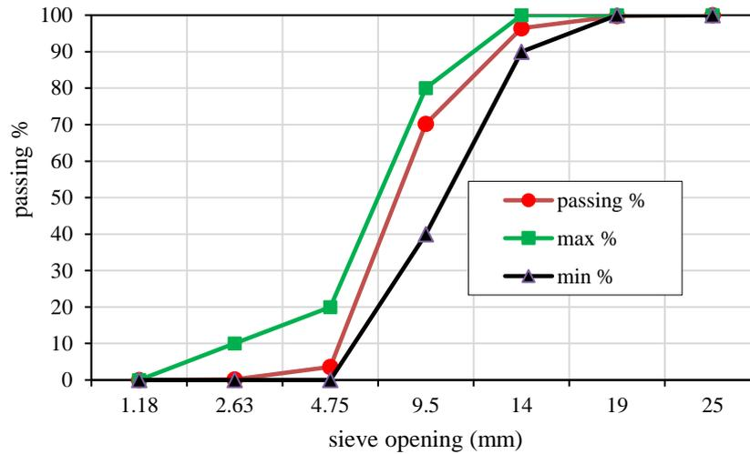
Fig. 4. Grading curve of lightweight aggregate
