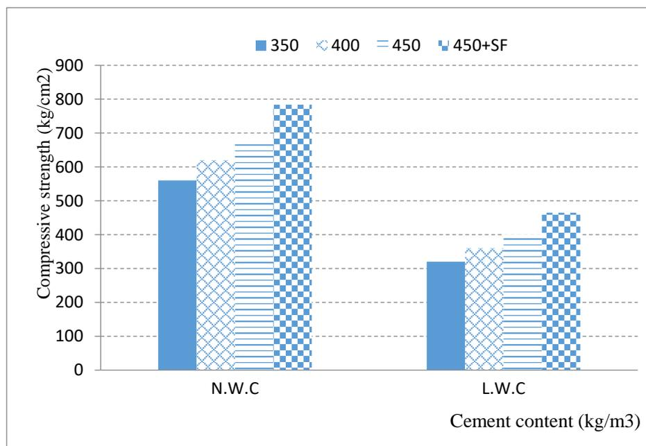
Fig. 10. Effect of cement content and silica fume on compressive strength of concrete cubes (350 kg/m<sup>3</sup>, 400 kg/m<sup>3</sup> and 450 kg/m<sup>3</sup> cement content).
