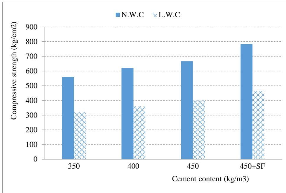
**Fig.8. Effect of concrete type on the compressive strength of concrete cubes (350 kg/m<sup>3</sup>, 400 kg/m<sup>3</sup> and 450 kg/m<sup>3</sup> cement content).**
