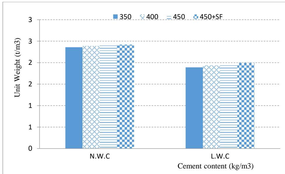
Fig. 11. Effect of cement content and silica fume on the unit weight of concrete cubes (350 kg/m<sup>3</sup>, 400 kg/m<sup>3</sup> and 450 kg/m<sup>3</sup> cement content).
