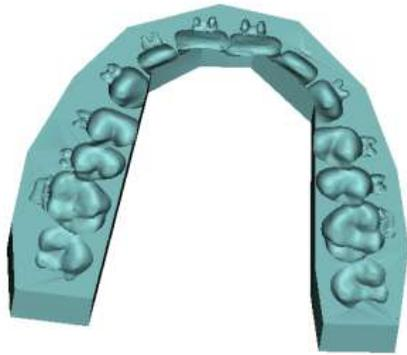
Fig5. Final shape of tray after subtraction teeth and bracket.
