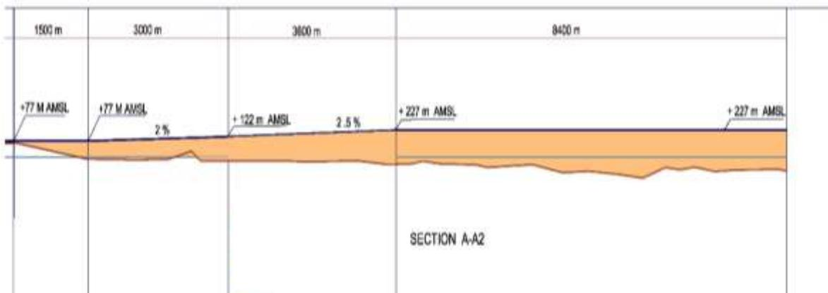
Fig. 11. Section A-A (Longitudinal section – Approach direction)
