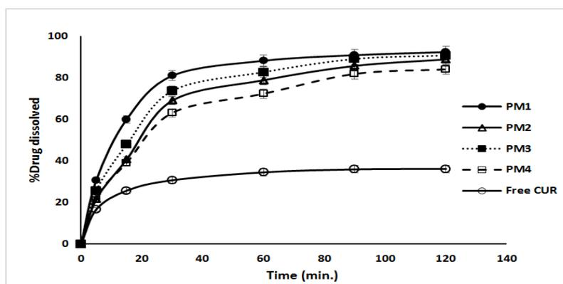
**Fig. 5:** Dissolution profile of the physical mixtures of curcumin with different combined stabilizers in phosphate buffer pH 4.7 and at 37 °C. The experiments were performed in triplicates and the mean  $\pm$ SD (n=3). (PM: physical mixture, CUR: curcumin).
