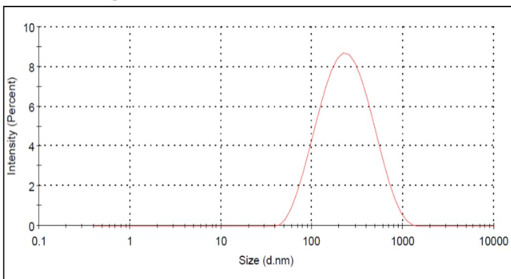
**Fig. 2:** Size distribution of the prepared nanocurcumin dispersion using PVP and PEG6000 combined stabilizers.
