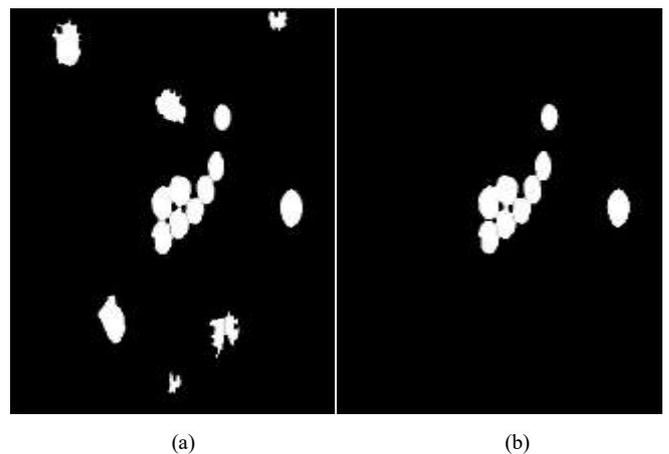
Fig. 9. (a) Border cleaning (b) Abnormal components removal
