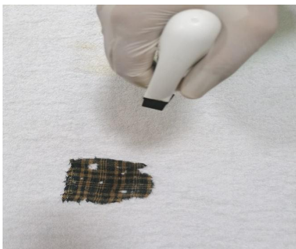
Fig. 12. Applying the nanocomposites by spraying on the artifact in the presence of a Teflon surface.
