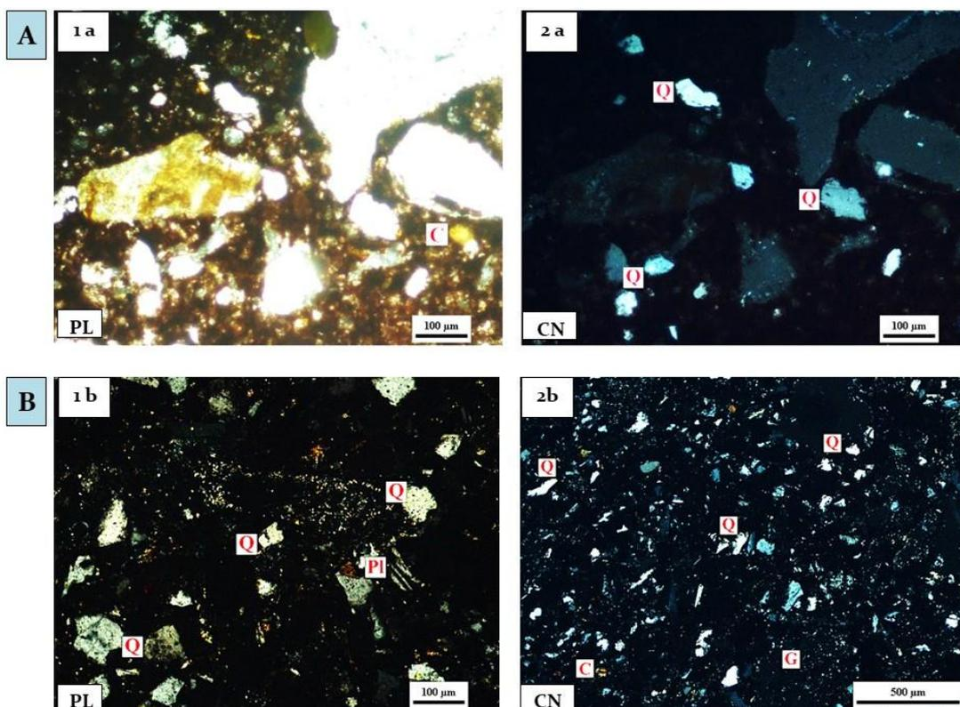
**Fig.4. Photomicrographs of thin sections of red brick sample1 shows the microfabrics of grains, (A) Calcite and quartz for sample (1), (B) Quartz, calcite, and Plagioclase is inside an iron-rich fabric in sample 2.**
