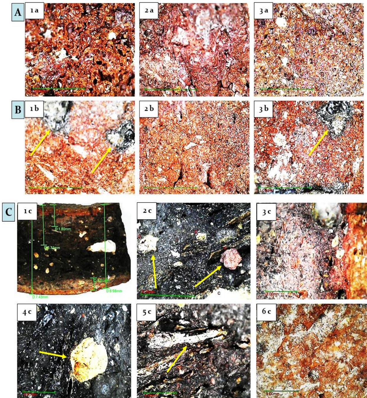
**Fig.3.** The investigation results of the samples by USB digital microscope. (A) Red brick from the lower part of the south wall, (B) Red brick from the north upper part of the small water tank, (C) The pottery water pipes used for the transportation of water among tanks.
