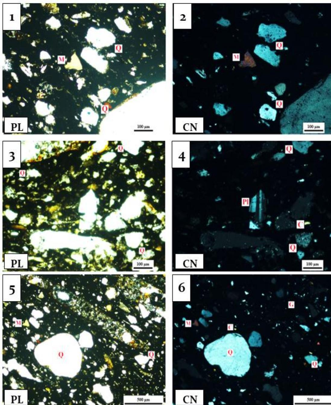
Fig. 5. Photomicrographs of thin sections of pottery water pipes show quartz(Q), calcite (C), plagioclase (PL), muscovite(M) and Grog(G).
