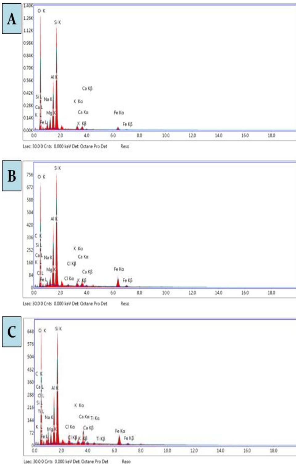
**Fig. 8.** EDX analysis results of the studied samples. (A, B) EDX spectra of the samples 1&2 of red bricks show that they consist of Si, Al, Na, Mg, Cl, K, Ca, C and Fe elements. (C) The sample of water pipes showed the same elements as the burnt bricks in addition to a high percentage of Ca element.
