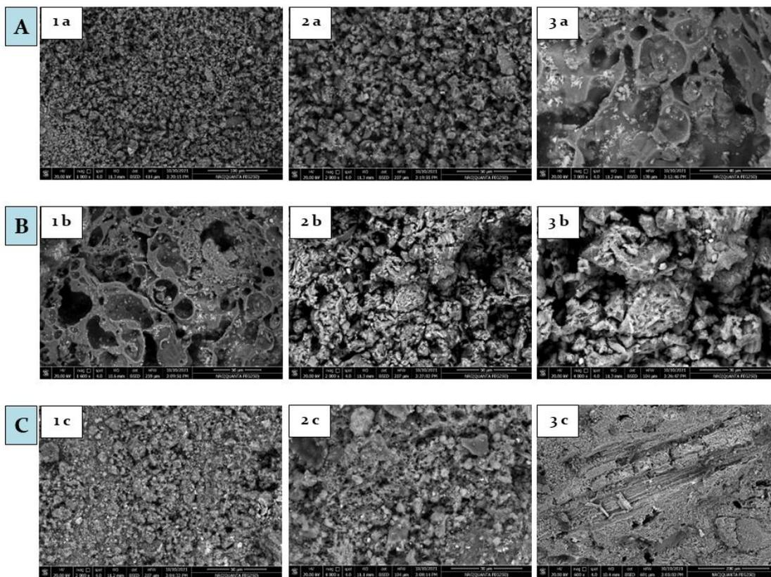
**Fig. 7. SEM micrographs of the samples, (A, B) Red brick ,(C) Water pottery pipes.**
