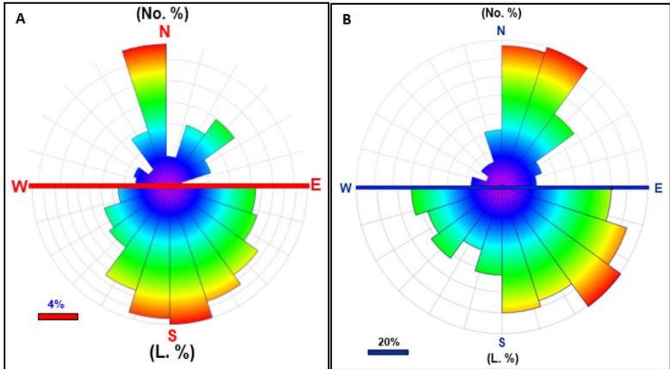
**Fig. 14.** Rose diagrams displaying the master trends of number (N) and length (L) proportions of surface lineaments: A) In the Dara area and B) In the Um Balad area.
