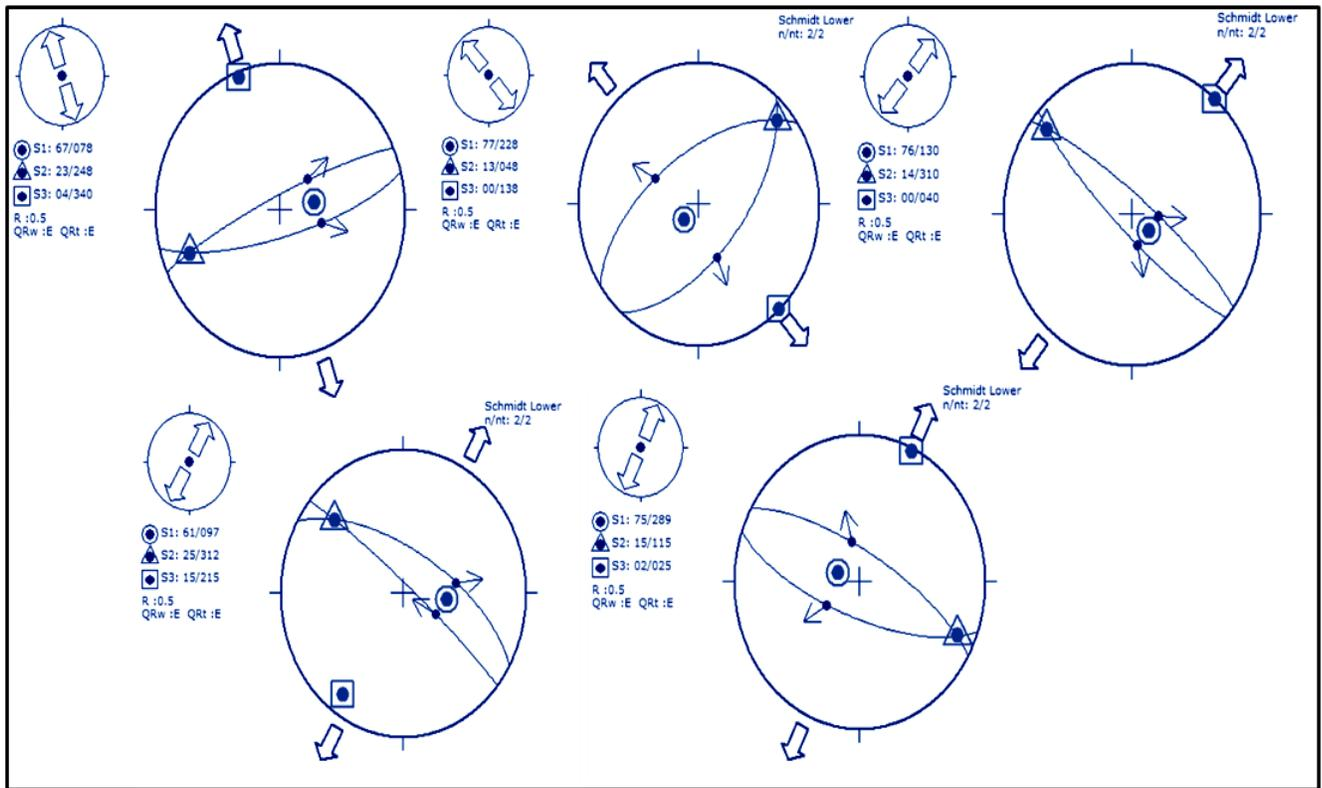
**Fig. 10.** Three principle stress axes of the two major conjugate sets for tension joints in the monzogranite of Dara mine area.
