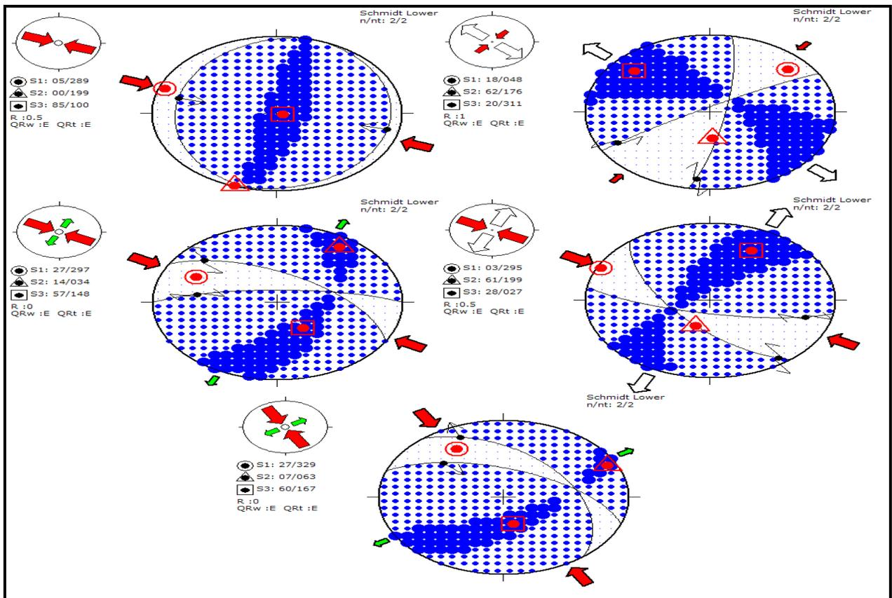
**Fig. 9.** Three principal stress axes of the two major conjugate sets for shear joints in the metagabbro-diorite of Um Balad area.
