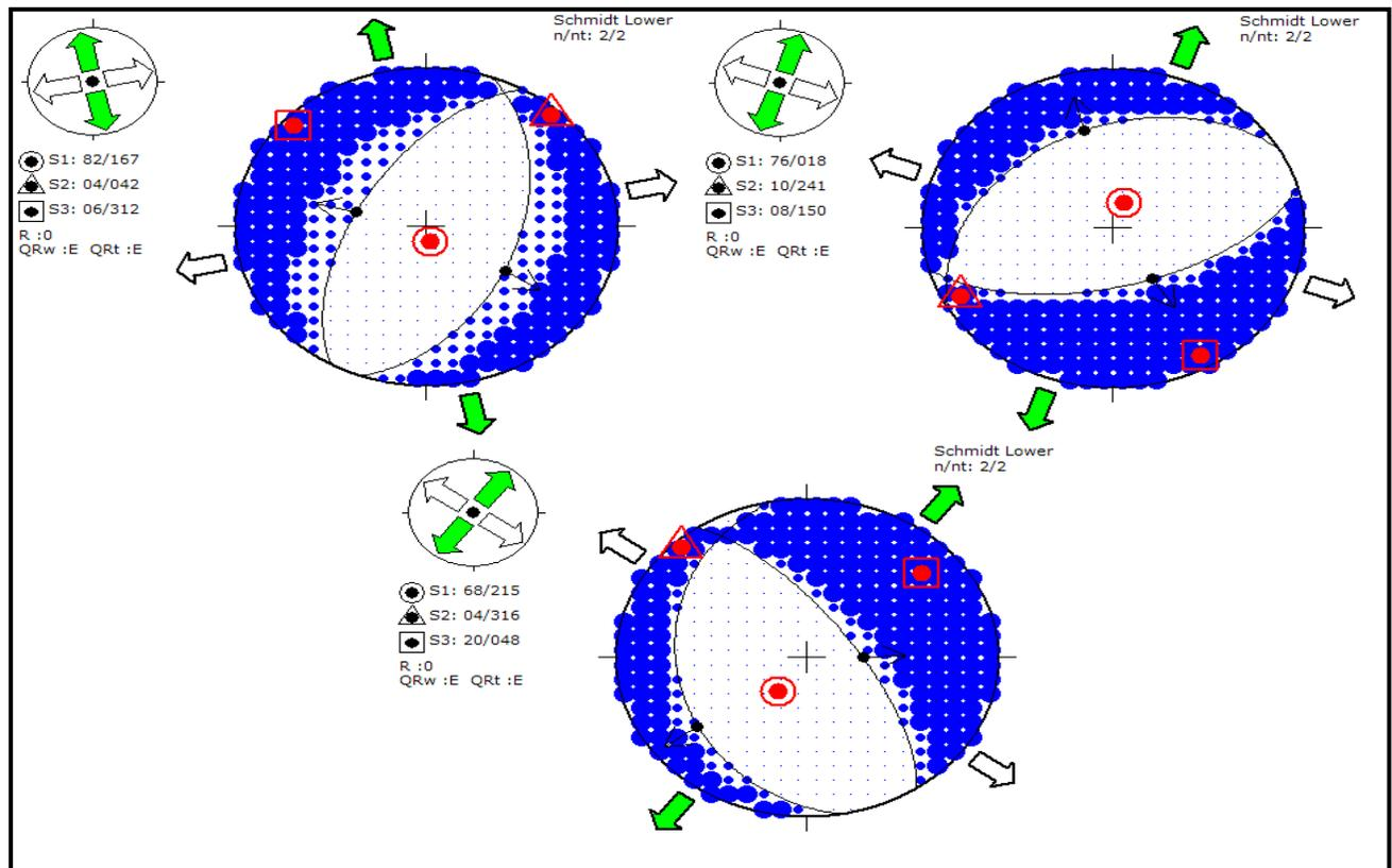
**Fig. 11.** Three principle stress axes of the two major conjugate sets for tension joints in the metagabbro-diorite of Um Balad area.
