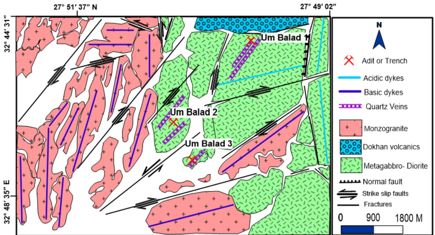
Fig. 6. Geologic-Structure map of the Um Balad mine area.
