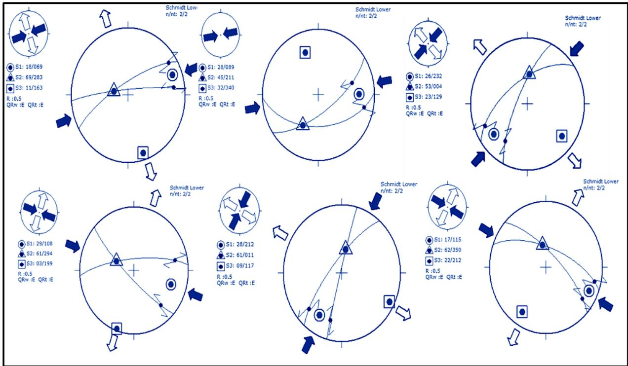
**Fig. 8.** Three principle stress axes of the two major conjugate sets for shear joints in the metagabbro-diorite of Dara area.
