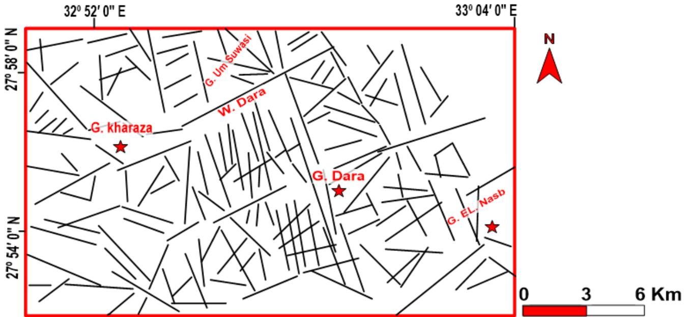
**Fig. 12.** Lineament map showing the distribution of structural lineaments in the Dara area.
