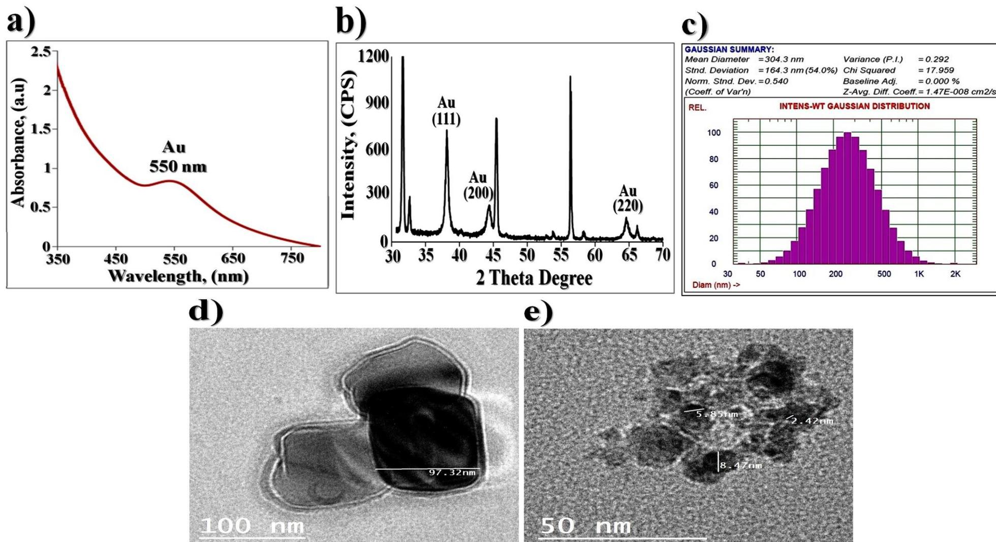
**Fig. 1.** Characterization of the synthesized gold nanoparticles (Au-NPs) showing **a)** Ultraviolet-visible (UV-VIS) spectroscopy, **b)** X-Ray Diffraction (XRD) spectrum, **c)** Dynamic Light Scattering (DLS), **d)** Transmission Electron Microscope (TEM) image of Au-NPs and **e)** TEM image of Au-NPs incorporated into *N. oculata* algal extract.
