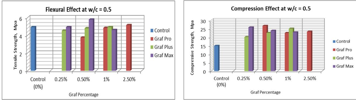
Figure 17: Flexural & Compressive Strength of Tested specimens at w/c=0.5
