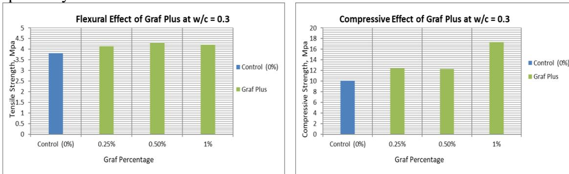
**Figure 7: Flexural and Compressive Strength of Tested Specimens strengthened with Graf Plus at w/c=0.3**
