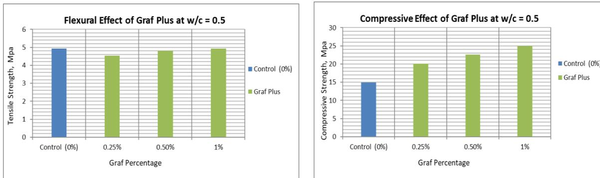
**Figure 15: Flexural and Compressive Strength of Tested Specimens strengthened with Graf Plus at w/c=0.5**
