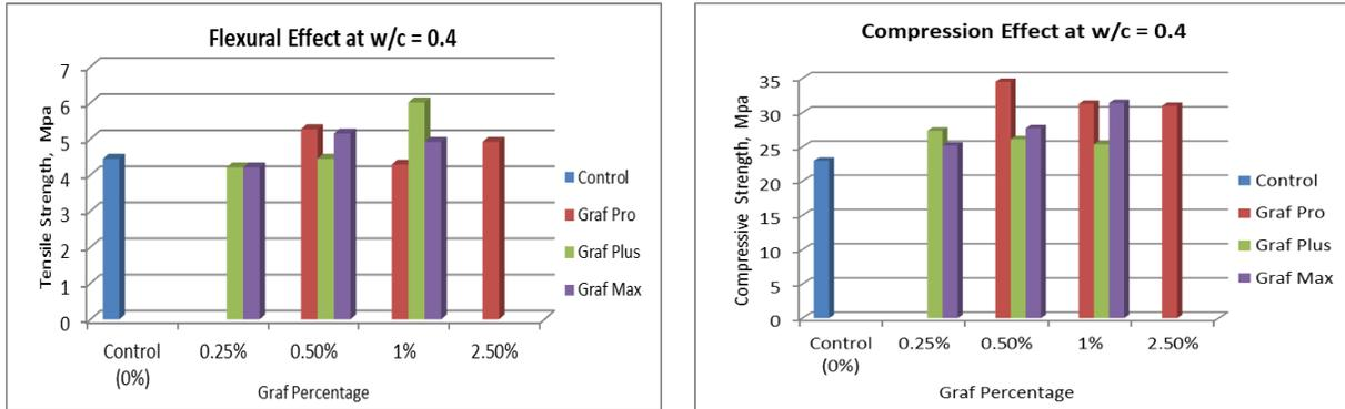
**Figure 13: Flexural & Compressive Strength of Tested specimens at w/c=0.4**
