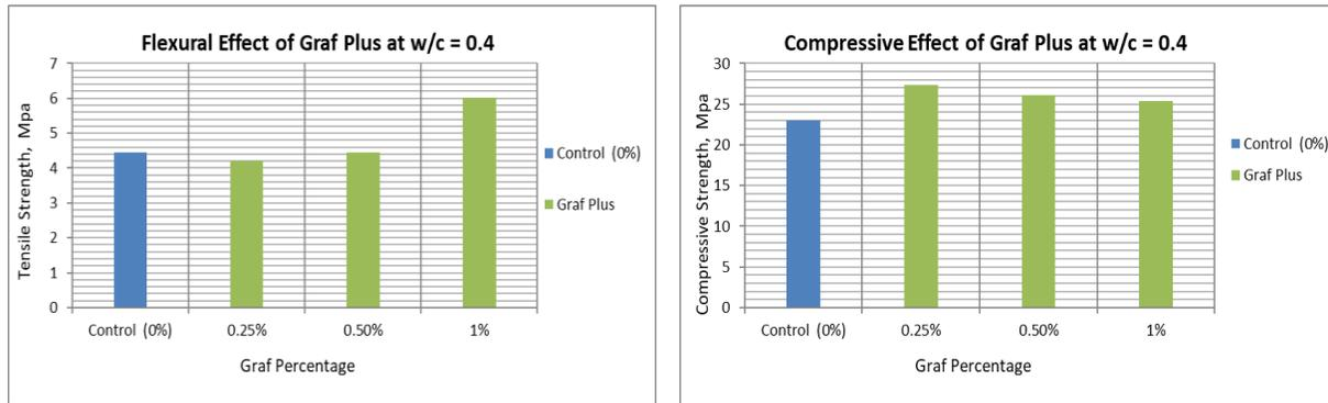
**Figure 11: Flexural and Compressive Strength of Tested Specimens strengthened with Graf Plus at w/c=0.4**
