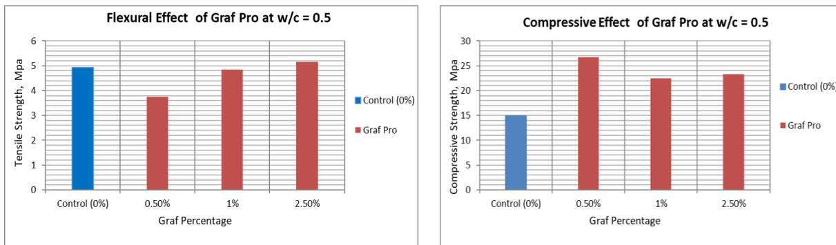
**Figure 14: Flexural and Compressive Strength of Tested Specimens strengthened with Graf Pro at w/c=0.5**
