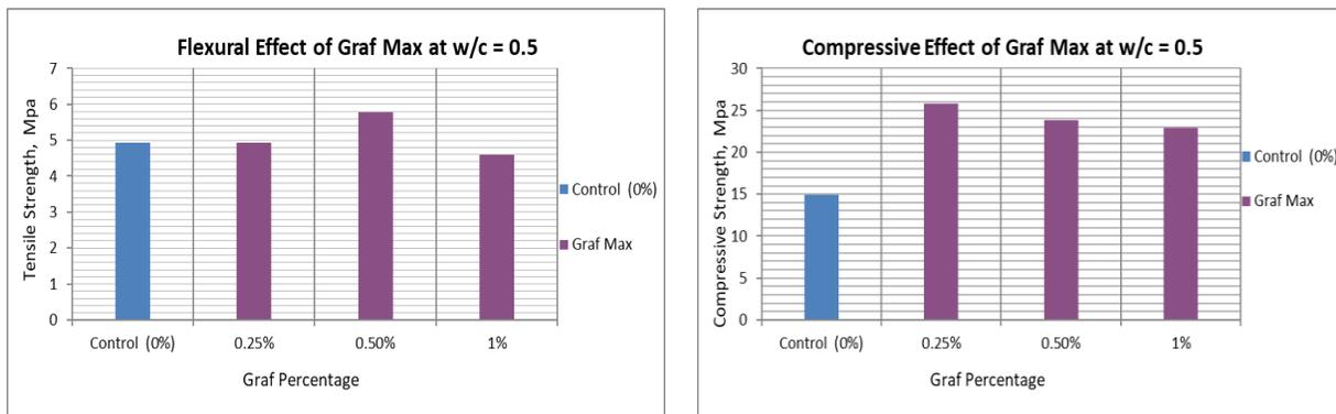
**Figure 16: Flexural and Compressive Strength of Tested Specimens strengthened with Graf Max at w/c=0.4**
