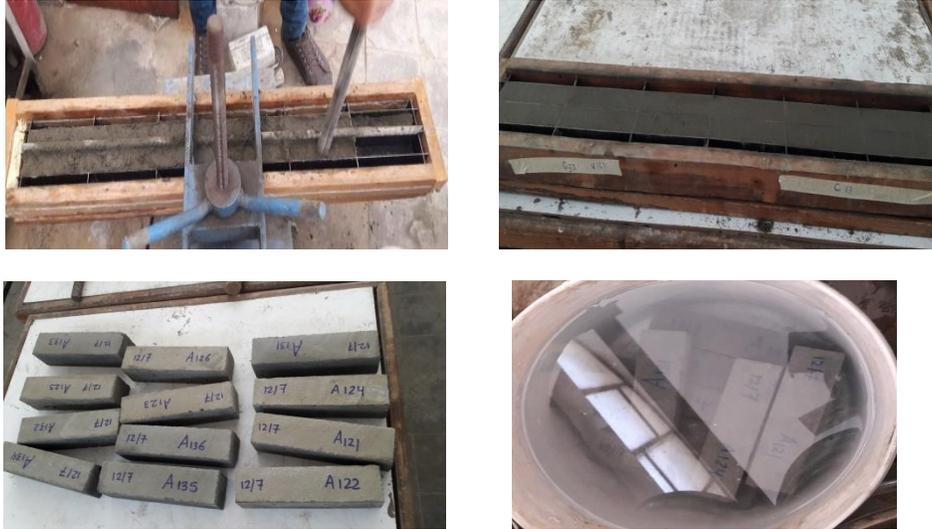
**Figure 2: The tested specimens during casting and curing**
