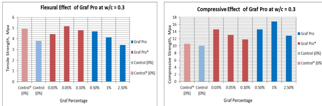
Figure 5: Flexural and Compressive Strength of Tested Specimens strengthened with Graf Pro at w/c=0.3
