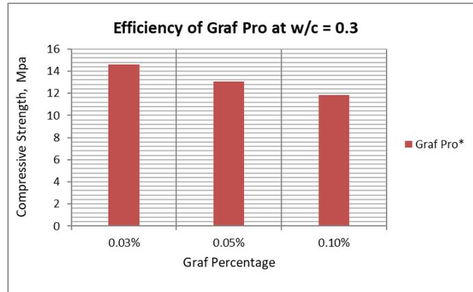
**Figure 6: Effect of increasing Graf Pro Ratio on Compressive Strength**
