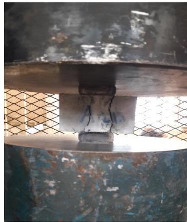
**Figure 3: Test set up for flexural & compression of tested specimens According to ESS 2421-7/2005**
