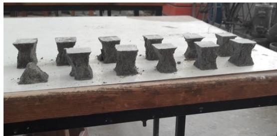
**Figure 4: Failure mode of tested specimens containing different nano particles**
