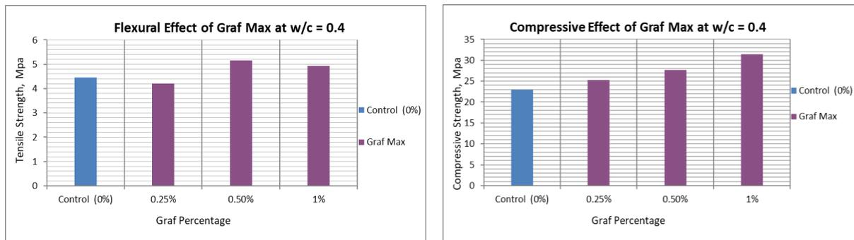
**Figure 12: Flexural and Compressive Strength of Tested Specimens strengthened with Graf Max at w/c=0.4**
