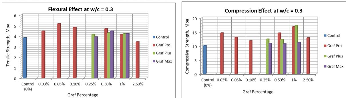
**Figure 9: Flexural & Compressive Strength of Tested specimens at w/c=0.3**
