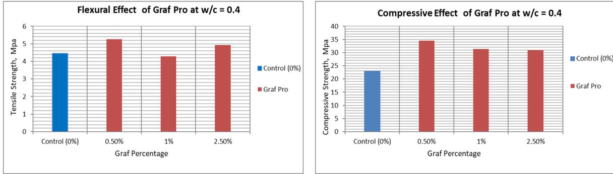
**Figure 10: Flexural and Compressive Strength of Tested Specimens strengthened with Graf Pro at w/c=0.4**
