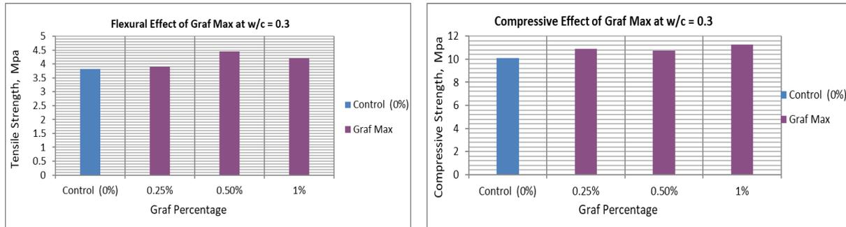
**Figure 8: Flexural and Compressive Strength of Tested Specimens strengthened with Graf Max at w/c=0.3**
