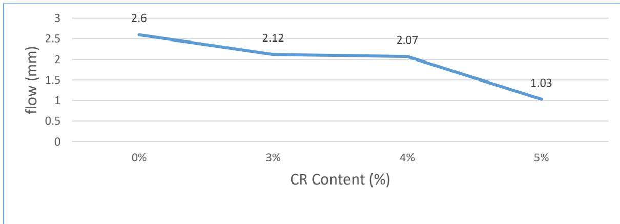
**Figure (4): Flow for MCM with 40% RCA & Different Percentages of CR by weight of asphalt binder**
