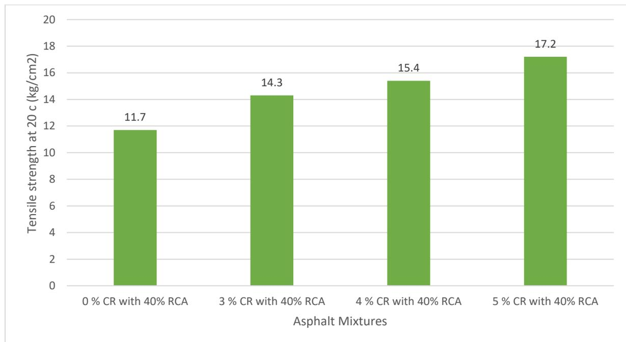
**Figure (9): The tensile strength at 20 C as indicator for asphalt mixture's fatigue**
