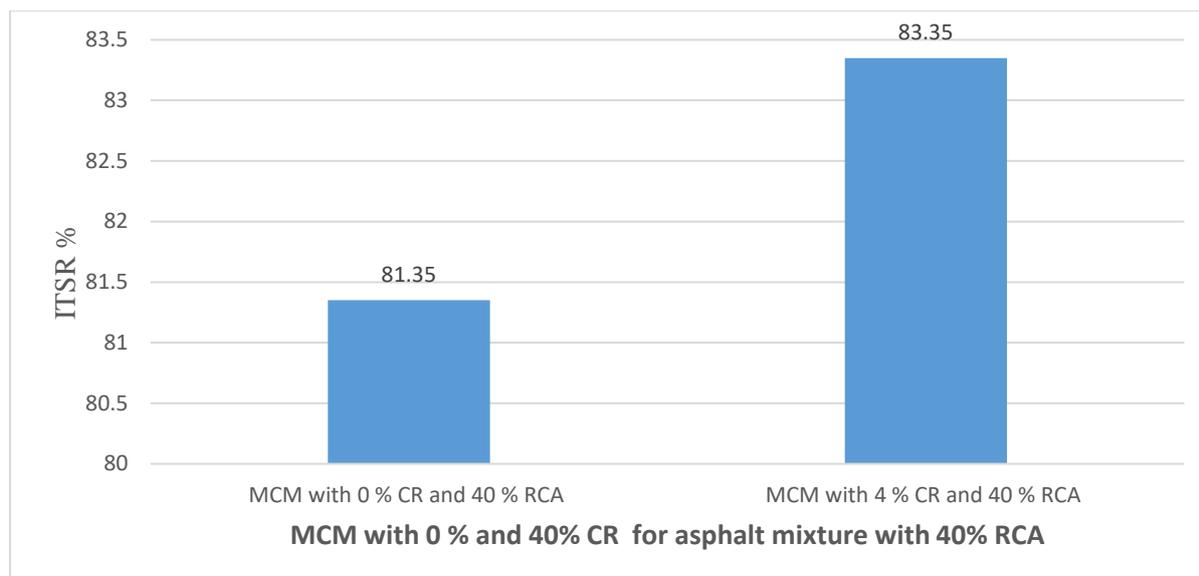
**Figure (7): Percentage of Indirect Tensile Strength Ratio ITSR (%) for MCM with 40% RCA and MCM with 40% RCA & 4 % CR**
