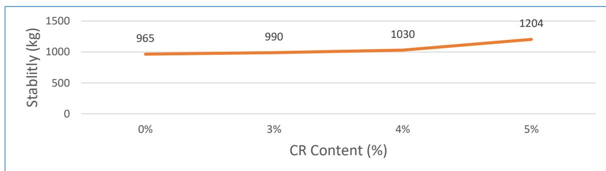
**Figure (3): Stability for MCM with 40% RCA & Different percentages of CR by weight of asphalt binder**
