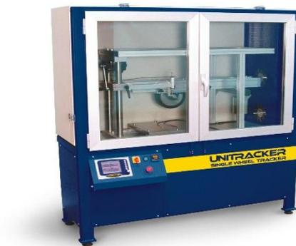
**Figure (2): Rutting Test Machine**
