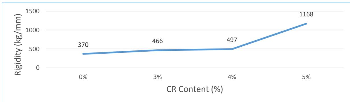
**Figure (5): Rigidity for MCM with 40% RCA by weight of aggregate & Different Percentages of CR by weight of asphalt binder**
