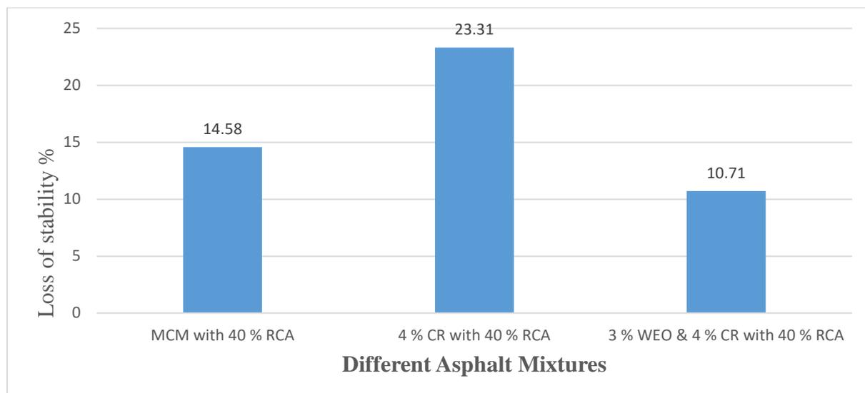
**Figure (10): Shows the results of loss of stability (%) for the different mixtures**
