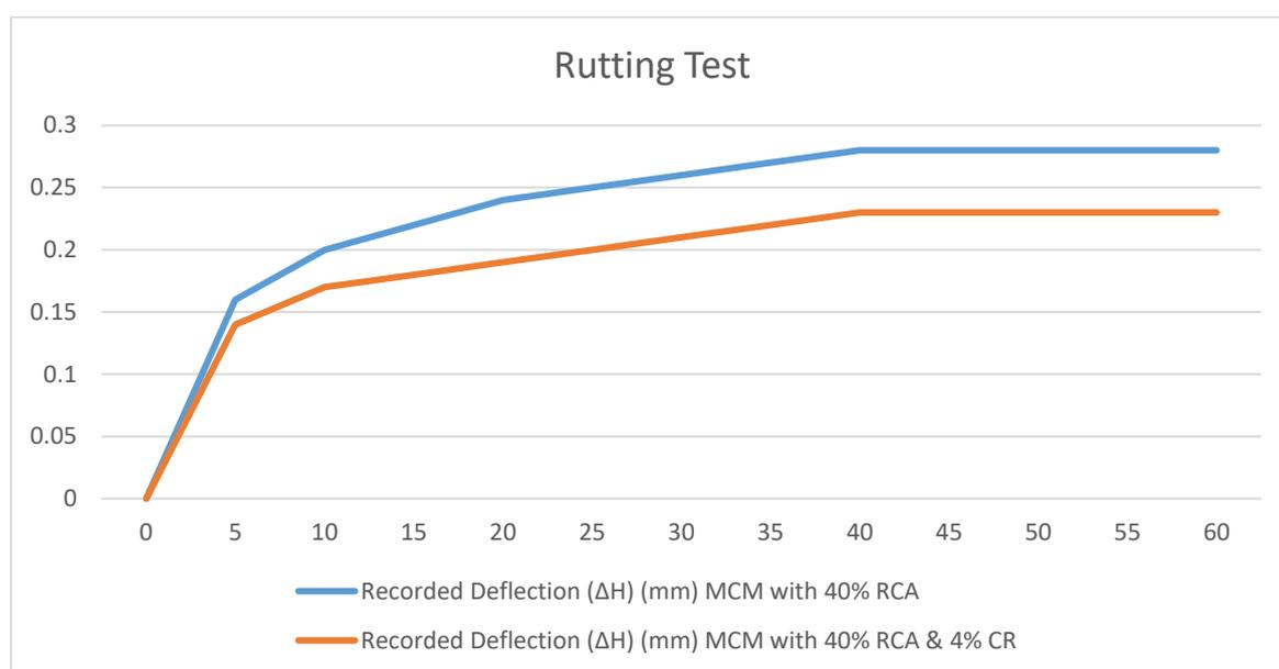
**Figure (8): Permanent Deformation Test (Rutting Test) Results (Deflection versus time) for MCM with 40% RCA and MCM with 40%RCA & 4% CR**
