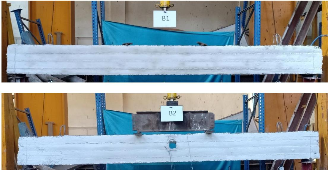
**Figure (5):** The Test Setup for the Prestressed beam.
