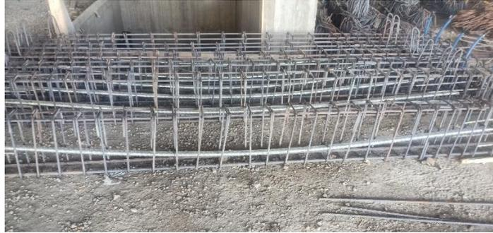
**Figure 6:** Preparation of tested samples Reinforcement
