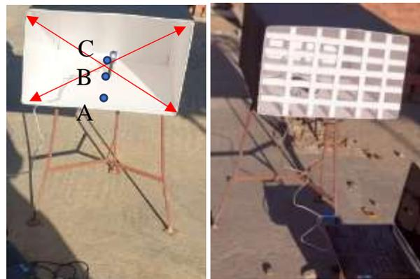
Figure 4 photos of the physical model; A: Model without shading A, B, C are the tested points, B: Model with shading system includes one layer (Source: researcher).
