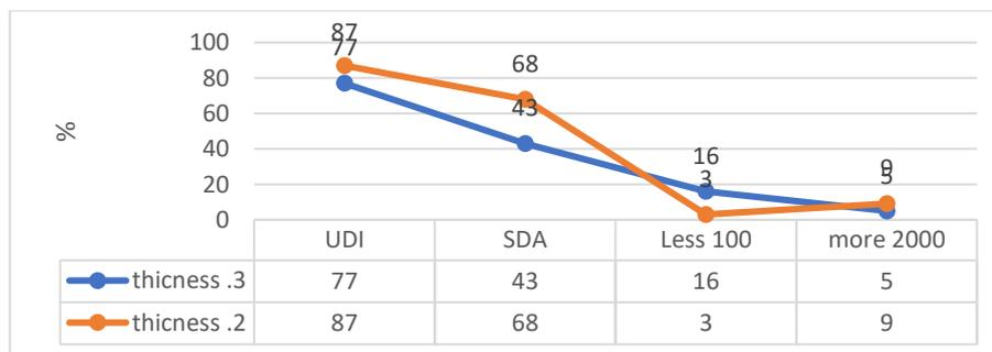
Figure 9 UDI and sDA for the pattern with one layer, it is simulated for three different thicknesses; 0.2m, 0.3m thicknesses (Source: researcher).
