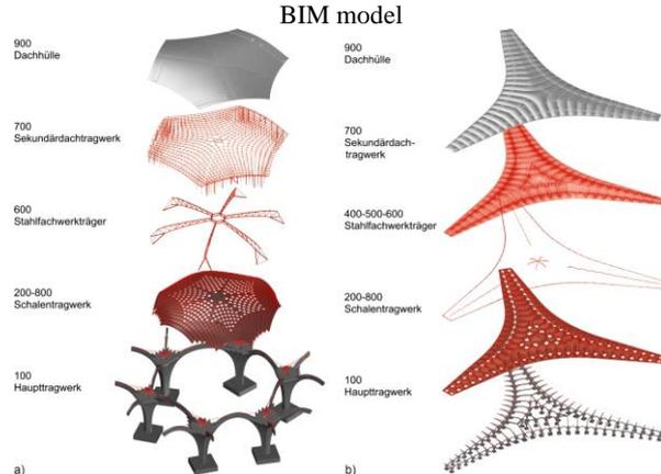
Figure 3 a) The individual components of the roof and primary structure in the central area, b) Placement of the individual components in the overall context[66]
