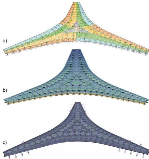
a) Central geometric digital model, b) FE model, c) BIM model
