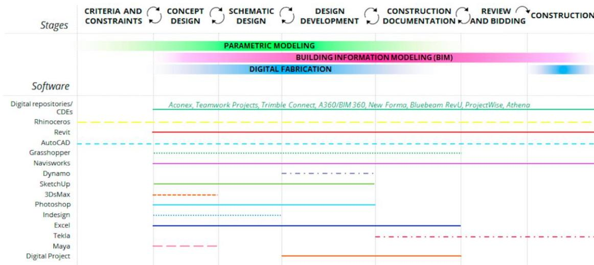
Figure (12) Presence of BIM, Parametric modeling, and digital fabrication, as well as the main software, pointed out by participants in the integrated design process stages.
