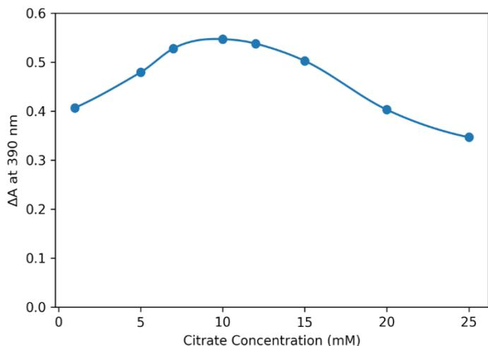
**Figure 3:** Effect of citrate concentration on  $\Delta A$  at 390 nm. Pregabalin concentration is  $300 \mu\text{g mL}^{-1}$  prepared in acetate buffer pH 3.8.
