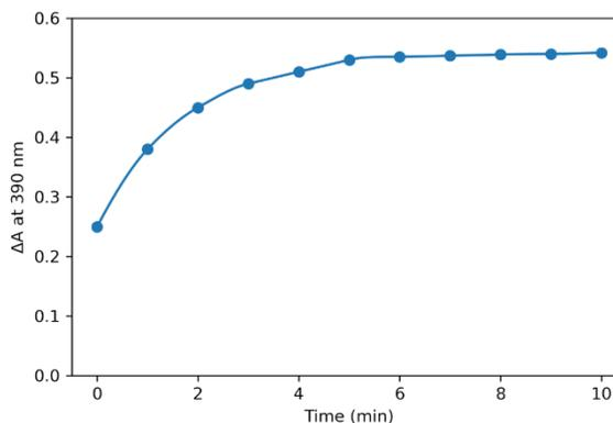
**Figure 8:** Effect of reaction time on  $\Delta A$  at 390 nm. Pregabalin concentration is  $300 \mu\text{g mL}^{-1}$ .
