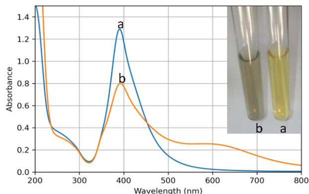
**Figure 1:** Surface plasmon resonance spectra and color of silver nanoparticles in (a) the absence and (b) the presence of  $300 \mu\text{g mL}^{-1}$  pregabalin.
