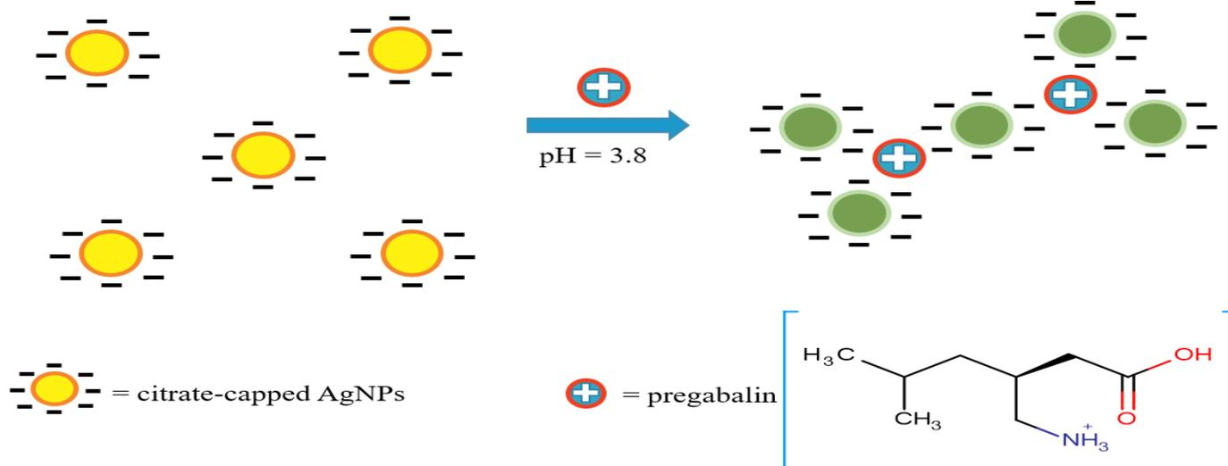
**Figure 2:** Schematic illustration of the colorimetric detection of pregabalin based on the aggregation of citrate-capped silver nanoparticles.
