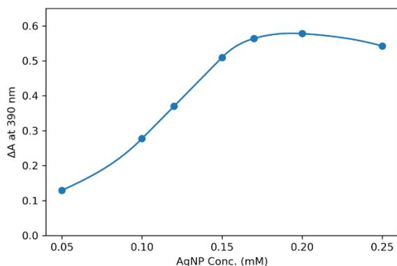
**Figure 7:** Effect of silver nanoparticles concentration on  $\Delta A$  at 390 nm. Pregabalin concentration is  $300 \mu\text{g mL}^{-1}$
