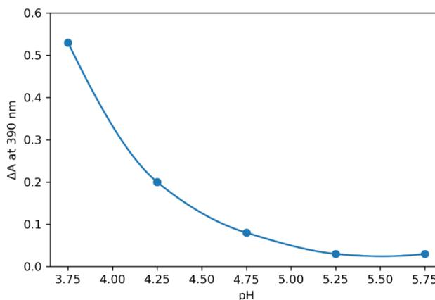
**Figure 5:** Effect of pH of acetate buffer on  $\Delta A$  at 390 nm. Pregabalin concentration is  $300 \mu\text{g mL}^{-1}$  prepared in acetate buffer.
