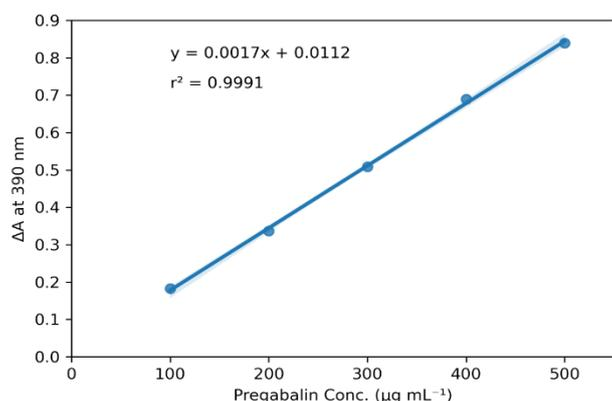
**Figure 10:** Calibration curve of pregabalin representing the linear relationship between  $\Delta A$  at 390 nm and pregabalin concentration.
