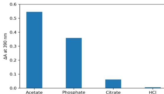
**Figure 4:** Effect of buffer type on  $\Delta A$  at 390 nm. Pregabalin concentration is  $300 \mu\text{g mL}^{-1}$  prepared in the corresponding buffer
