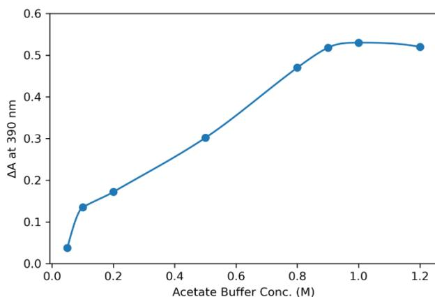
**Figure 6:** Effect of ionic strength of acetate buffer on  $\Delta A$  at 390 nm. Pregabalin concentration is  $300 \mu\text{g mL}^{-1}$  prepared in acetate buffer.
