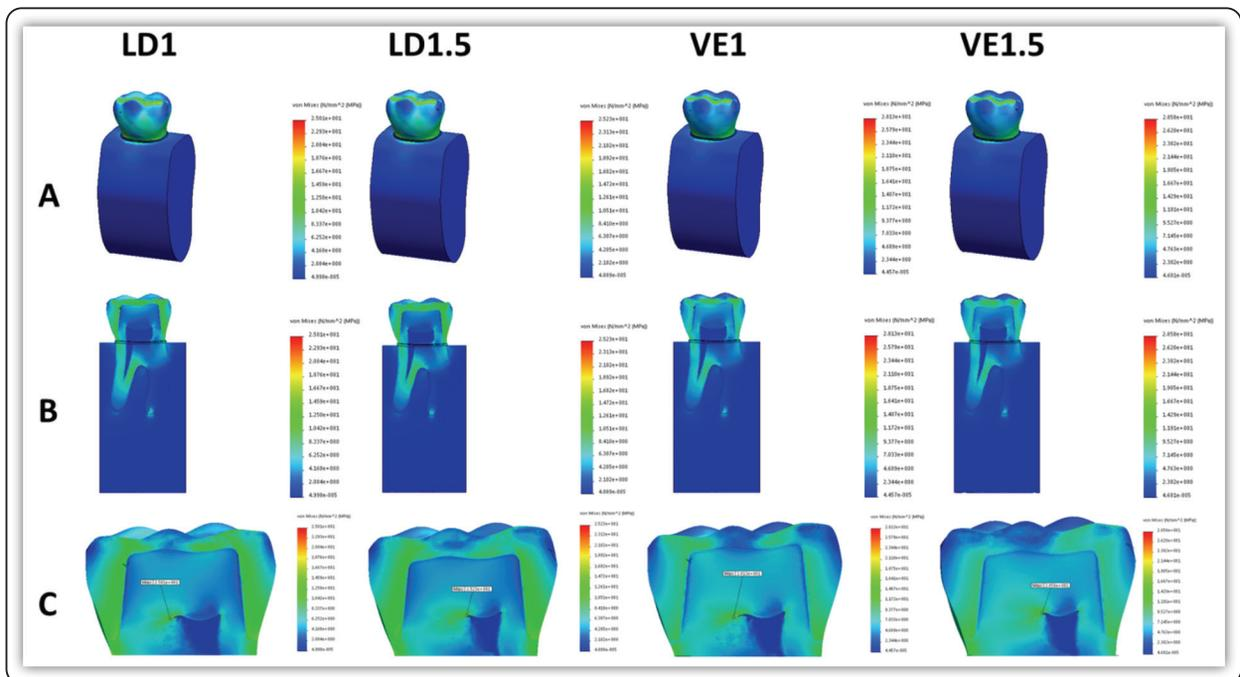
**FIG (2)** The resultant vMS distribution in the whole tested models; A: frontal view, B: sectioned view, C: area of highest vMS (demarcated)
