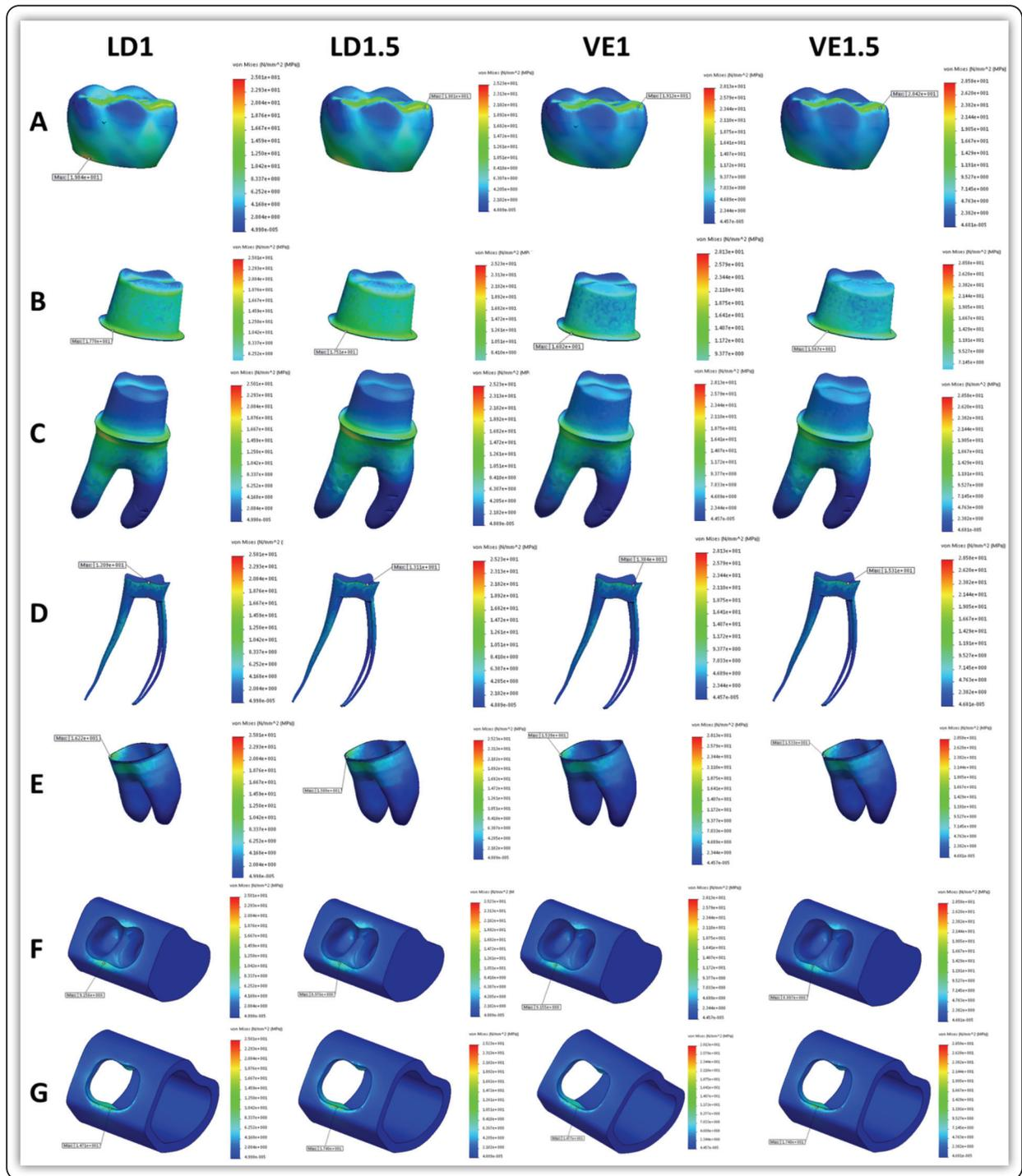
FIG (3) Stress distribution and areas of highest stress values within each part of the tested models; A: restoration B: cement layer, C: prepared tooth, D: pulp, E: periodontal ligament, F: cancellous bone, G: cortical bone
