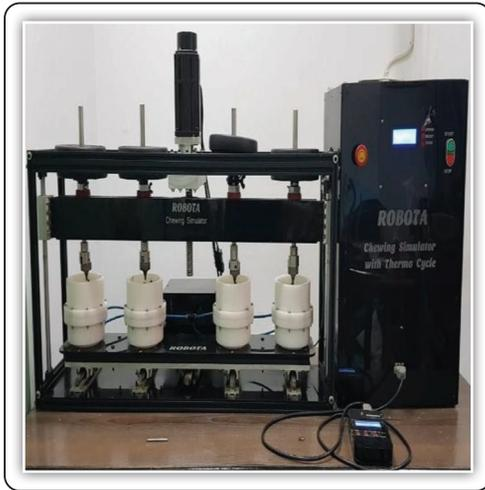
FIG (2) Each clasp and its models were mounted on the chewing simulator device.
