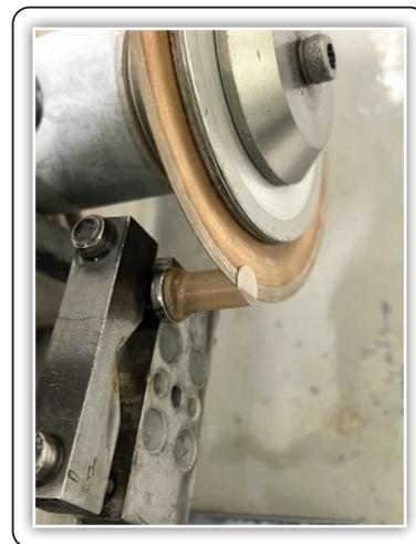
FIG (1) Isomet disc cutting ceramic disc
