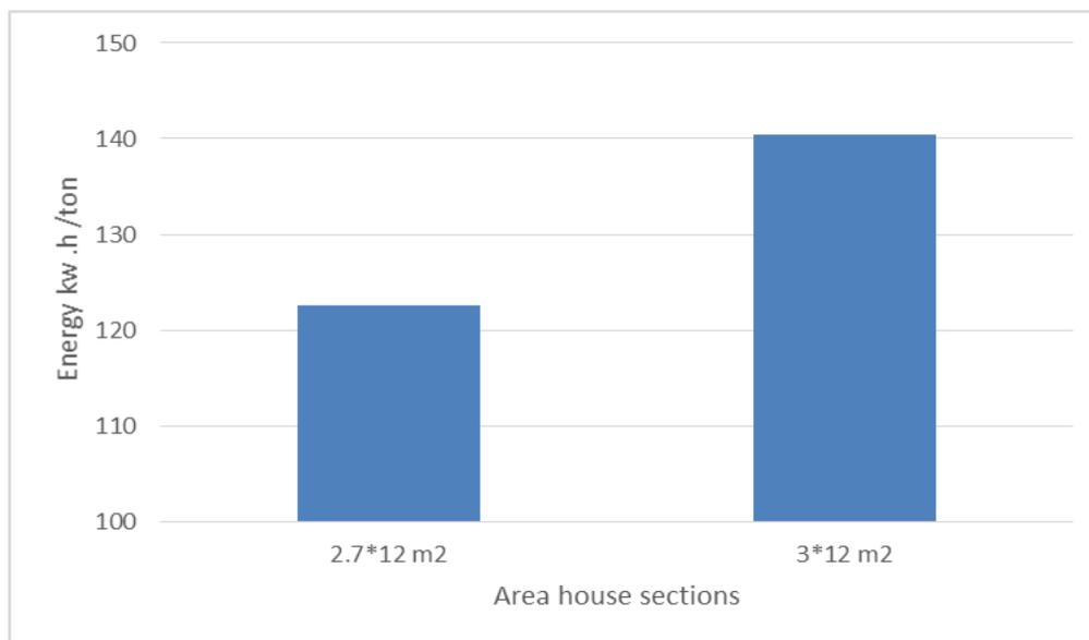
**Fig. 6. Effect of area house section on energy at constant ambient temperature of 28 C° and air velocity of 2.5 m/sec.**
