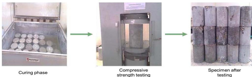
**Figure 22.** steps of concrete specimen from curing to testing and its final shape (Mangi, 2017)
