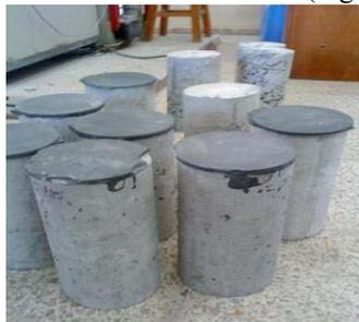
**Figure 18.** Concrete blocks after curing (Kumari, 2015)
