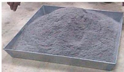
**Figure 21.** Bagasse ash after being burned in a close drum (Mangi, 2017)
