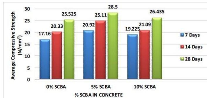
**Figure 23.** Compressive strength of concrete M20 mix with different SCBA percentages and different curing periods (Mangi,2017)
