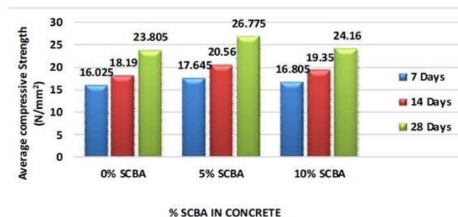
**Figure 24.** Compressive strength of concrete M15 mix with different SCBA percentages at different curing periods (Mangi, 2017)
