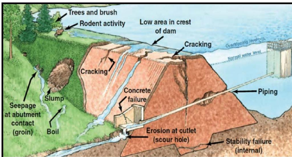
Figure (1) Various Reasons of Earth dam's Failure [8].
