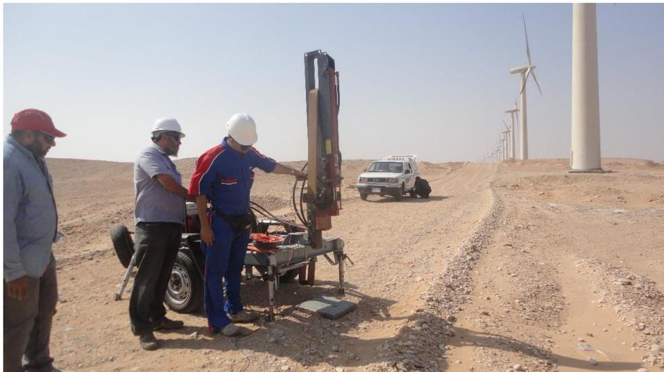
**Fig. (13)** A weight drop 150 kg is used
