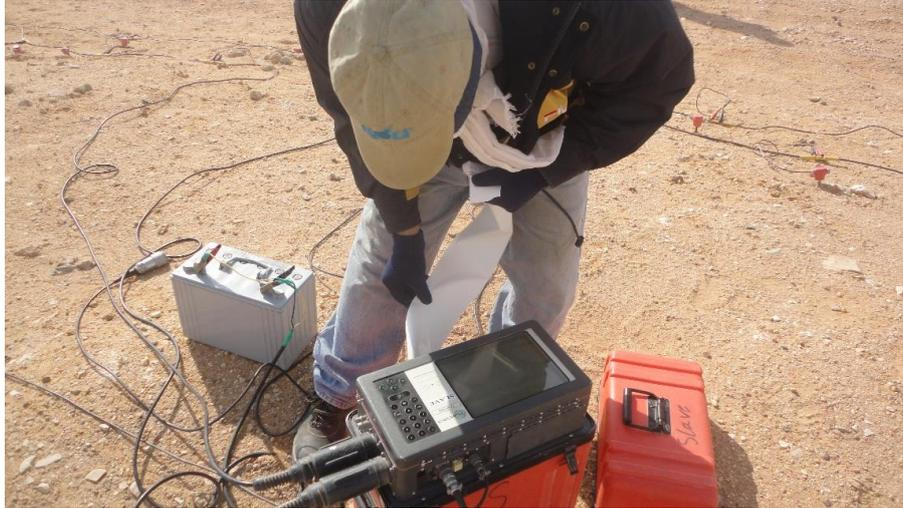
**Fig. (12)** The StrataView data logger which used in the shallow seismic refraction survey
