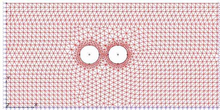
Fig. 3: 2-D finite element model of tunnel (new tunnel running side by side to existing tunnel)
