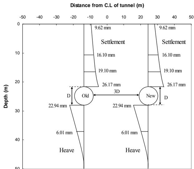
Fig. 7: Vertical displacement at different levels along centerline of twin tunnel with three-diameter horizontal separation
