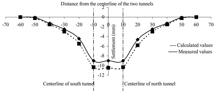
Fig. 5: Vertical displacement of soil at the ground surface after achievement of El-Azhar road tunnels construction (Case history)
