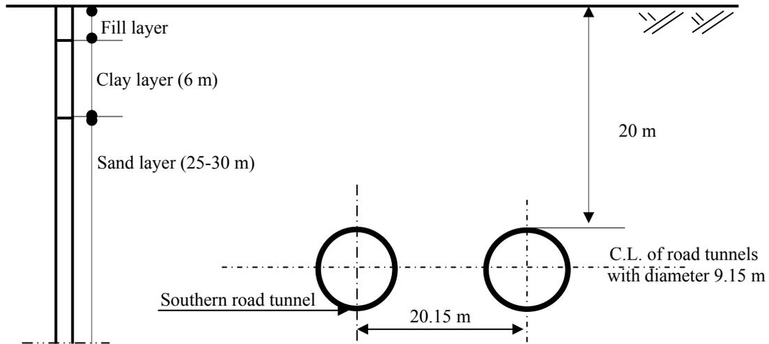
Fig. 2: Cross section along El-Azhar road tunnel (Case study)
