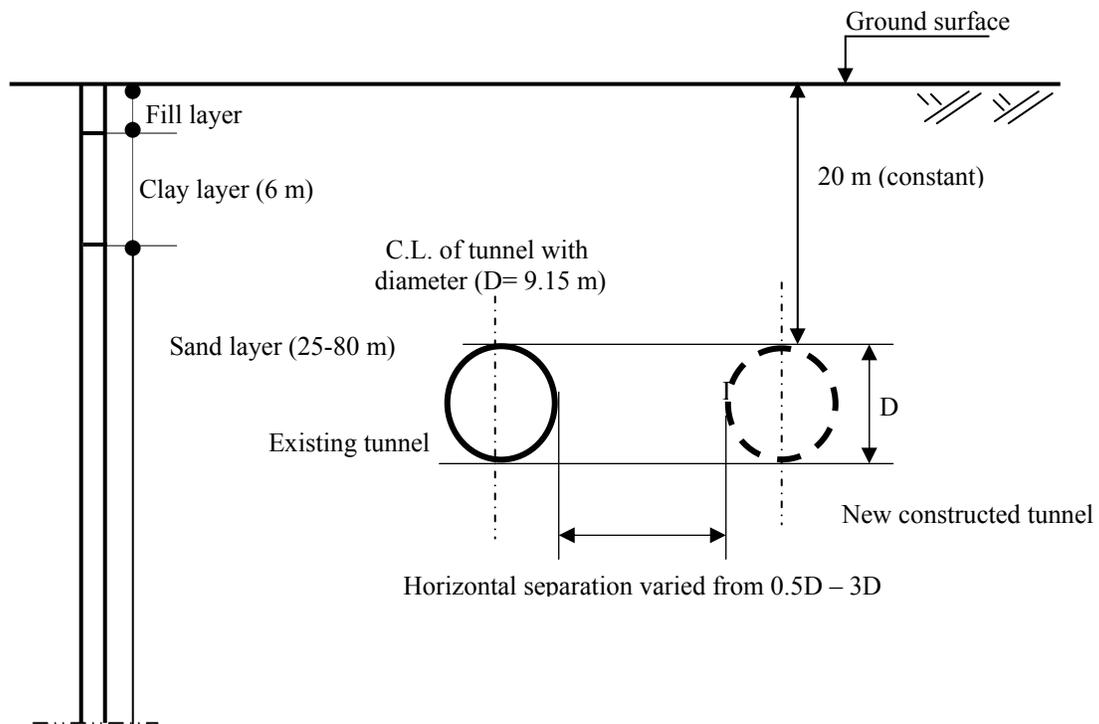
Fig. 1: Cross section showing the twin tunnels (parallel side-by-side)
