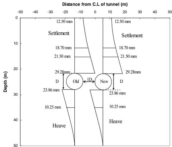
Fig. 6: Vertical displacement at different levels along centerline of twin tunnel with one-diameter horizontal separation
