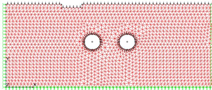
Fig. 4: 2-D finite element model of tunnel (case history- side by side)
