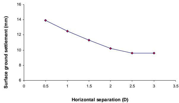
Fig. 8: Calculated settlement at ground surface with different horizontal separations (new tunnel running side-by-side old tunnel)
