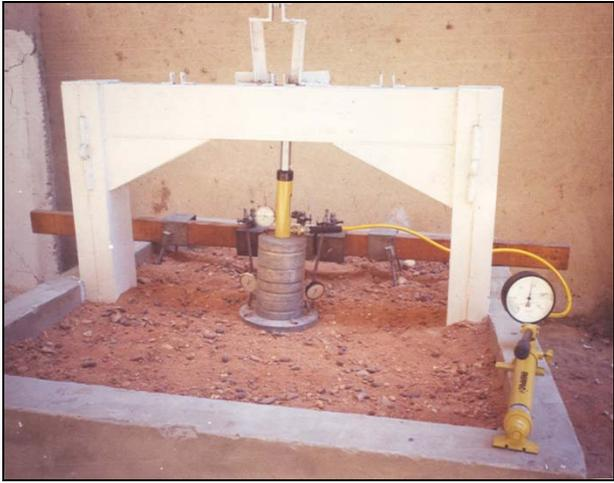
Figure (2): Plate loading test setup
