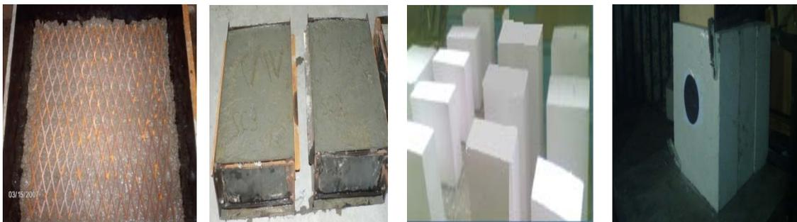
*Figure (1): square plain concrete and ferrocement specimens*
