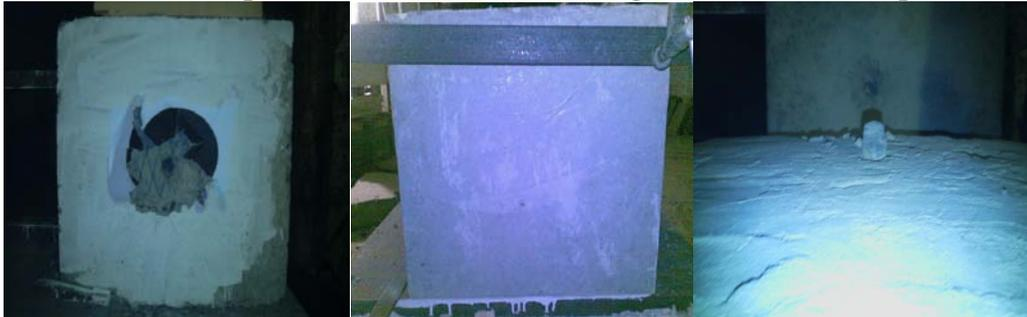
Damage in Front Face of ferrocement slab      Damage in rear Face of ferrocement slab      projectile stopped inside the panel
