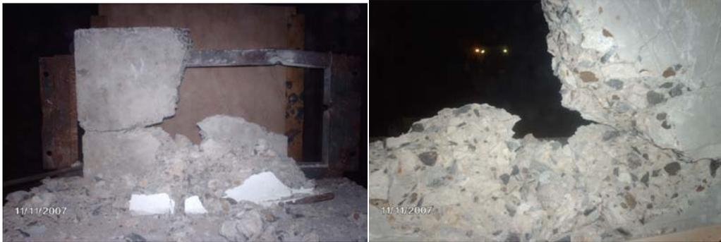
Damage in Front Face of plain concrete slab      Damage in rear Face of plain concrete slab
