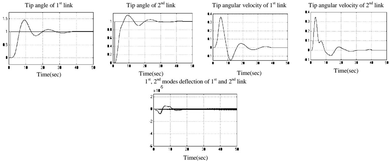
**Figure (10)** The simulation results of the fuzzy controller of non linear model of two flexible links.
