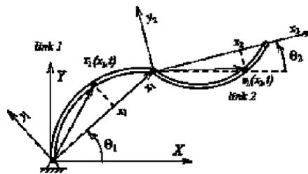
**Figure(1) The two flexible link robot**
