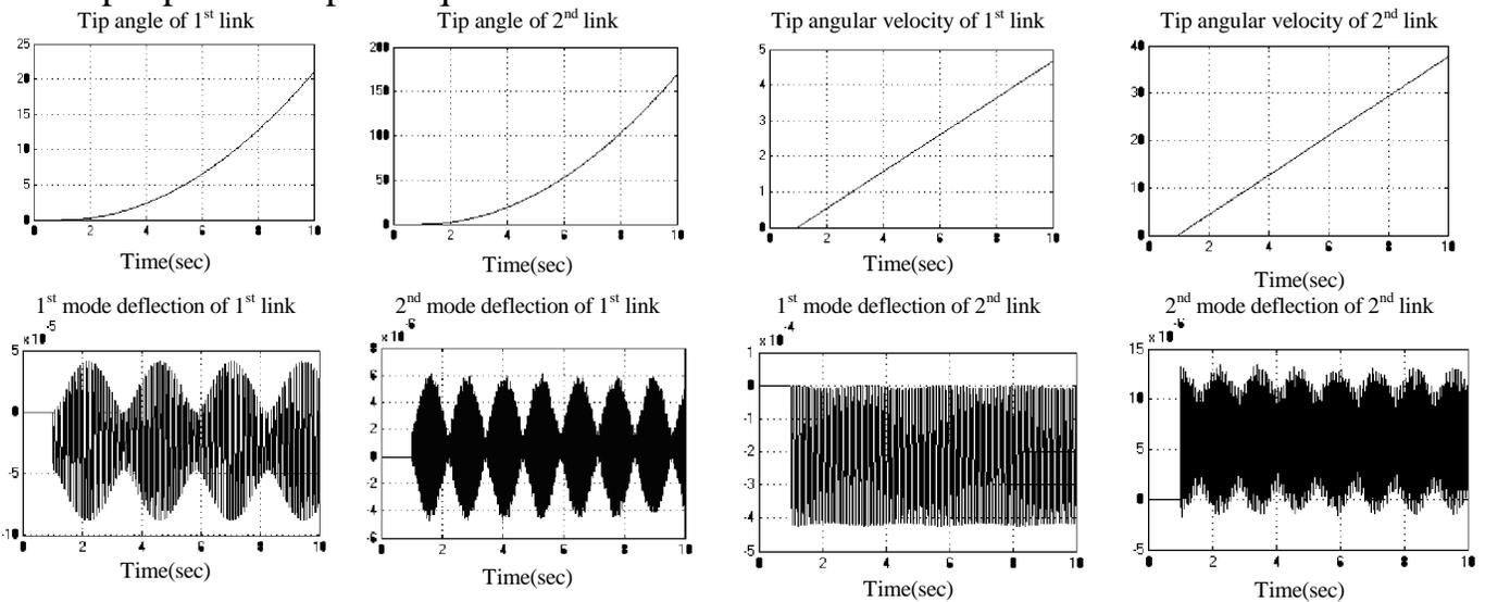
Figure (2) Simulation of open loop of linear model of two flexible links.
