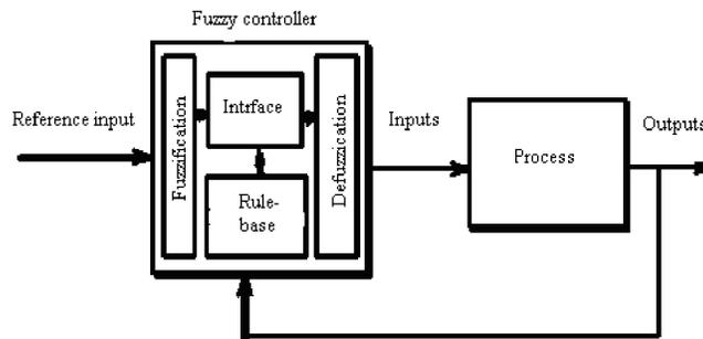
Figure (4) The basic configuration of the fuzzy system.
