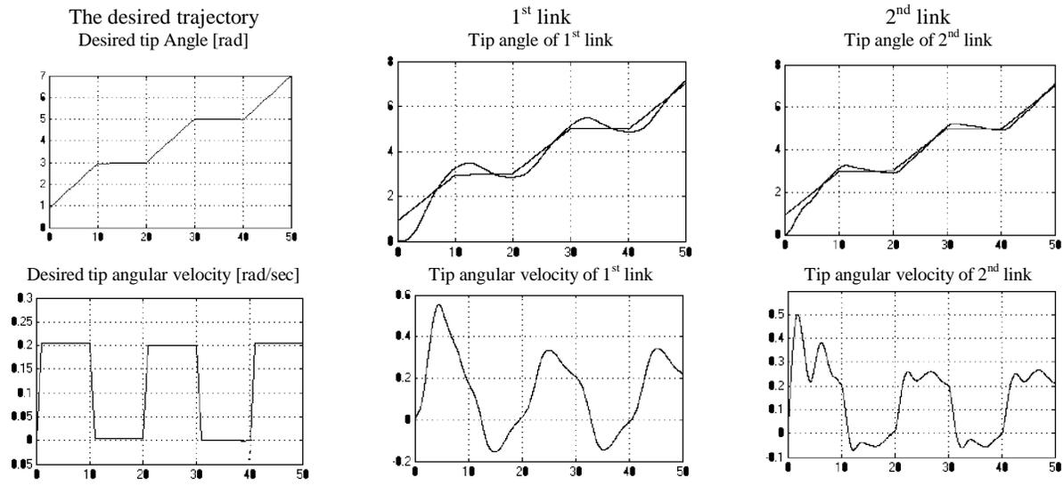
Figure (8) The simulation results of the desired trajectory of two flexible link
