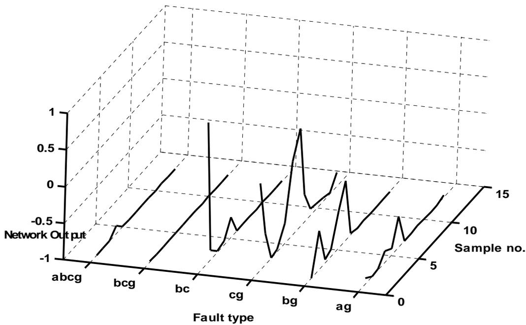
**Figure 5:** Fault location network output for faults at 20 miles, fault resistance 20  $\Omega$ , conduction angle 62°,  $\delta=-20^\circ$ , fault inception angle is 90°.
