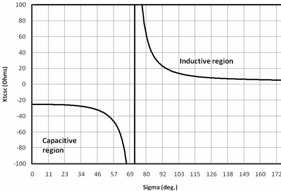
Figure (2): Impedance characteristics of the TCSC.
