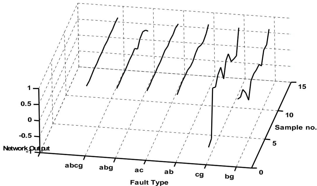
**Figure 6:** Fault location network output for faults at 100 miles, fault resistance 50  $\Omega$ , conduction angle 45°,  $\delta= -10^\circ$ , fault inception angle is 0°.
