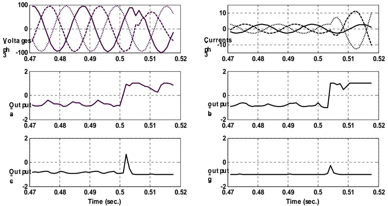
**Figure 4:** Fault classification network output for a-b fault at 90 miles, fault resistance  $50 \Omega$ , conduction angle  $50^\circ$ ,  $\delta = -10^\circ$ , fault inception angle is  $90^\circ$ .
