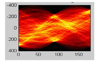
Fig.3 Hough transform of a sample hole defect
