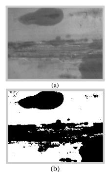
Fig.6 (a)original image of a rust defect (b)Global thresholded image of the rust defect
