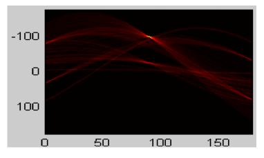
Fig.4 Hough transform of a sample scratch defect
