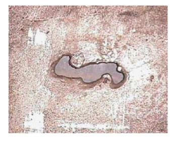
Fig.1 A sample of hole defect
