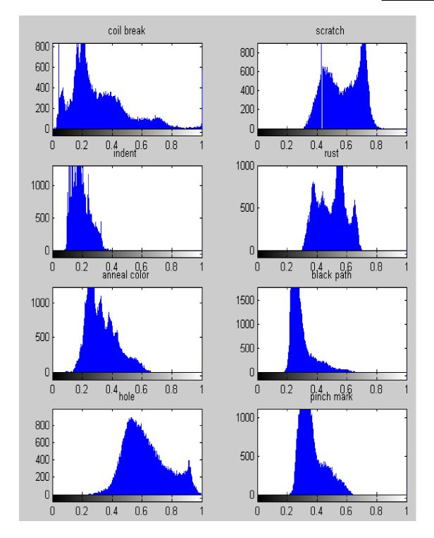
Fig.5 Comparisons of the coil break defect image histogram with the other defects
