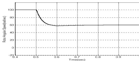
Fig6 Responses for a step decrease in speed reference amount to 40 rad/s , for initial steady state speeds of, (a) 180 rad/s ,(b) 100rad/s
