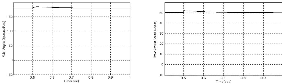
Fig.8 Responses for sudden unloading the motor from full-load to no-load torque, initial steady state speeds of ,(a) 180 rad/s, (b) 50 rad/s
