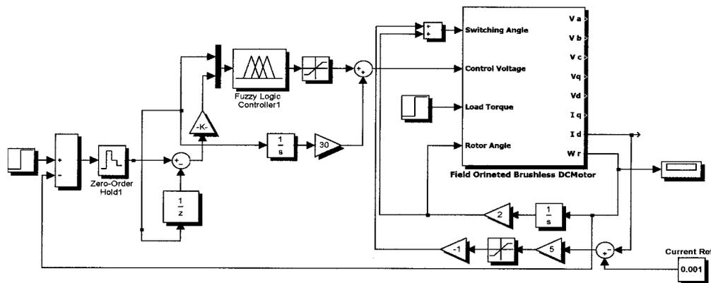
Fig. 1 The block diagram of the overall system
