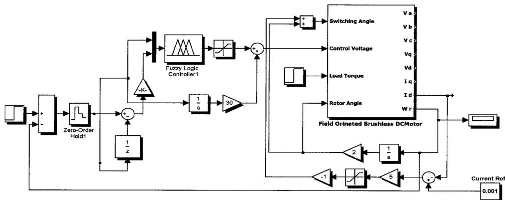
Fig. 3 The block diagram of the Brushless DC motor
