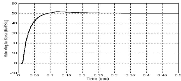
Fig. 5 Responses for step increase in speed reference from standstill with full-load torque supplied, (a)for 180rad/s (b)for 100 rad/s.
