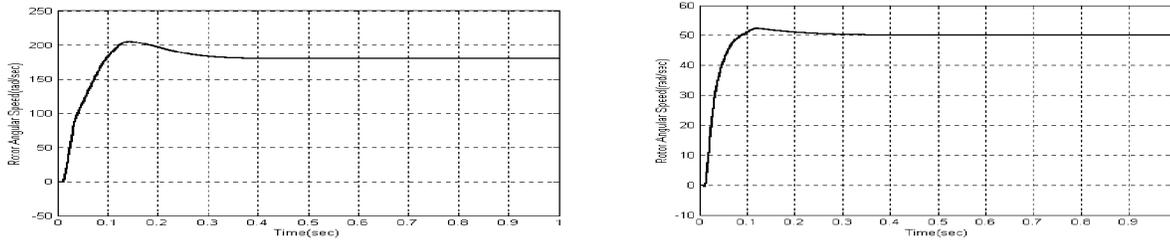
Fig. 7 responses of sudden increase in the speed reference from standstill with full-load torque supplied and for speed references of (a) 180 rad/s, (b) 50 rad/s.
