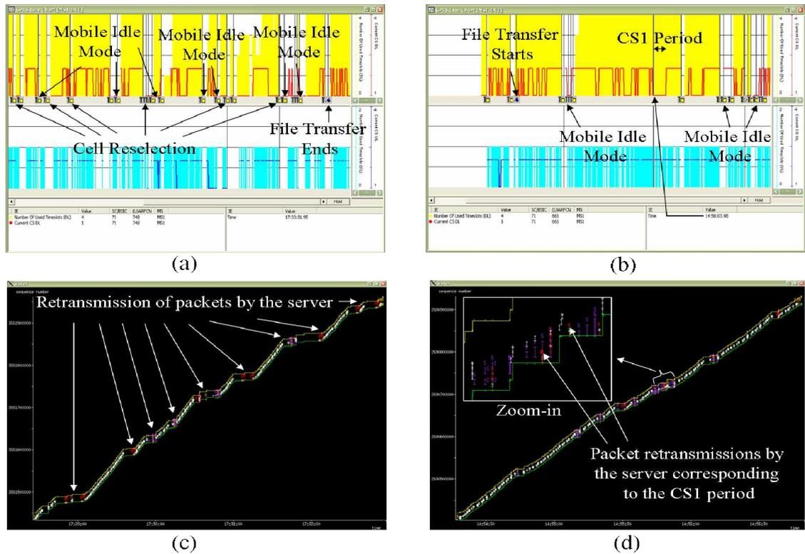
**Figure (5):** (a) Successive mobile idle mode and cell reselections (b) Prolonged bad channel condition (c) Successive retransmissions (R) (d) Retransmissions (R) during CS1 period
