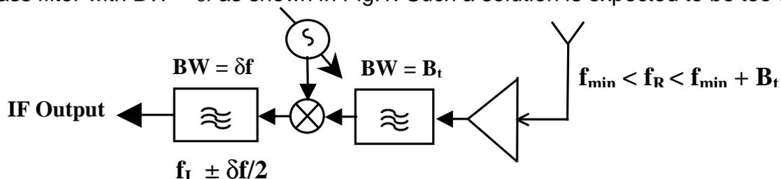
**Fig. 1. A simple scanning super-Heterodyne receiver**
