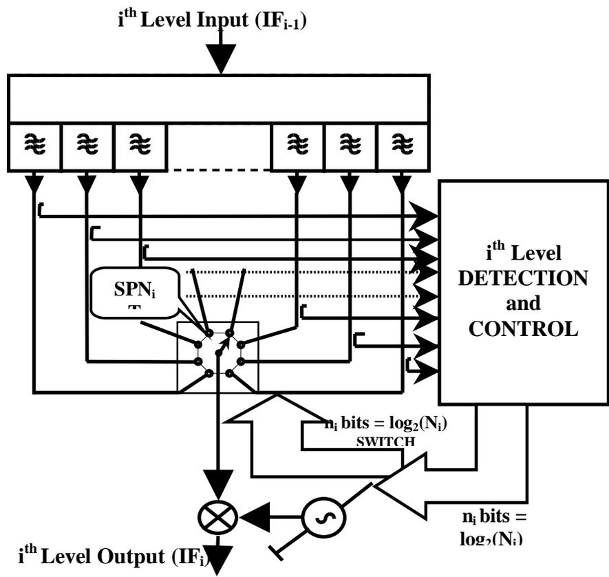
**Fig. 3. Functional Diagram of the  $i^{\text{th}}$  Channelization Level**
