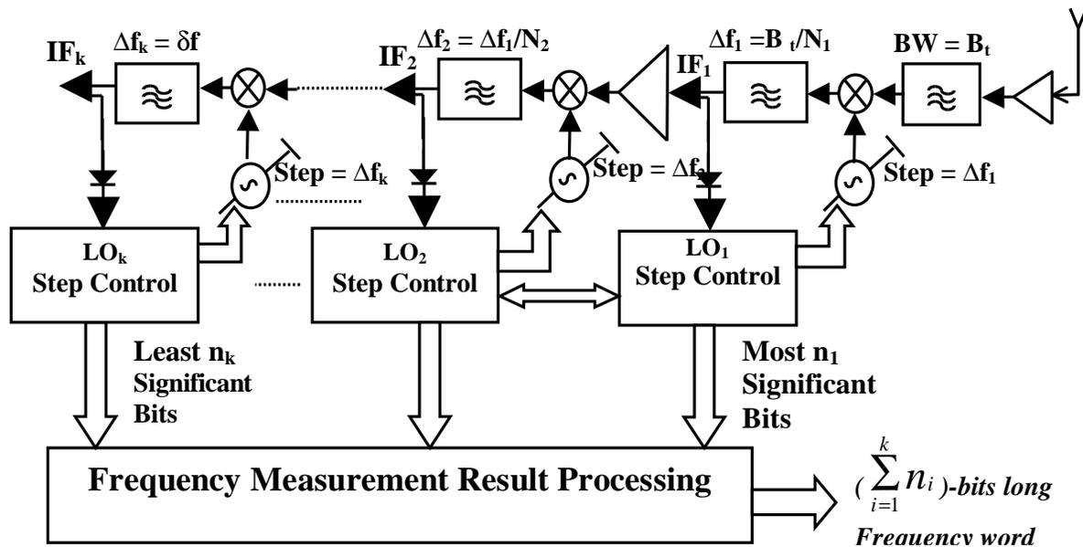
**Fig.2. A Proposed Multi-Level Scanning Super-Heterodyne**
