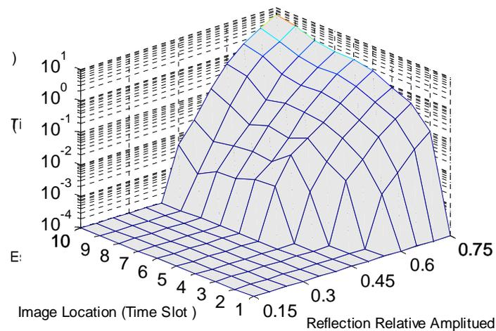
**Figure (6):** Estimated variance for different channel image amplitudes and locations using the proposed algorithm
