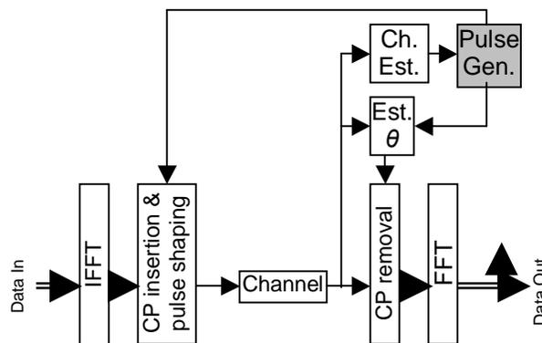
Figure (5): Adaptive pulse shaping system block diagram
