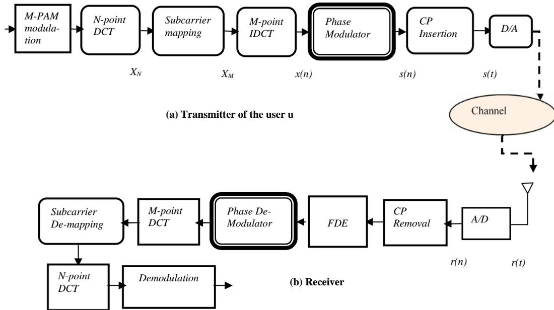
Figure (2): A block diagram of constant envelope DCT SC-FDMA-PM system over multipath channel.
