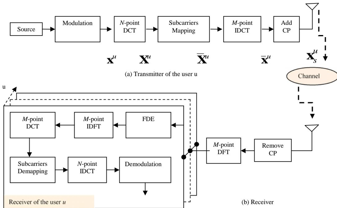
**Figure(1):** Structure of the DCT SC-FDMA system over a frequency selective channel.
