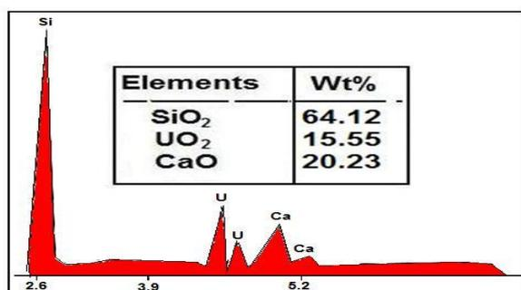
**Figure 18.** EDX chart for uranotile showing decreasing of UO<sub>2</sub> after treatment
