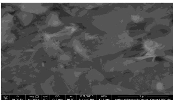
**Figure 17.** FIG image showing disappear bright color (uranotile) after treatment
