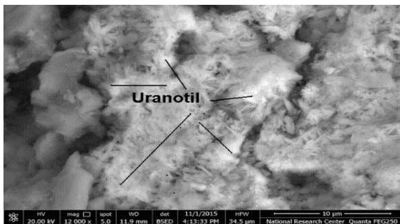
**Figure 15.** FIG image showing uranotile mineral before treatment by *Sargassum*
