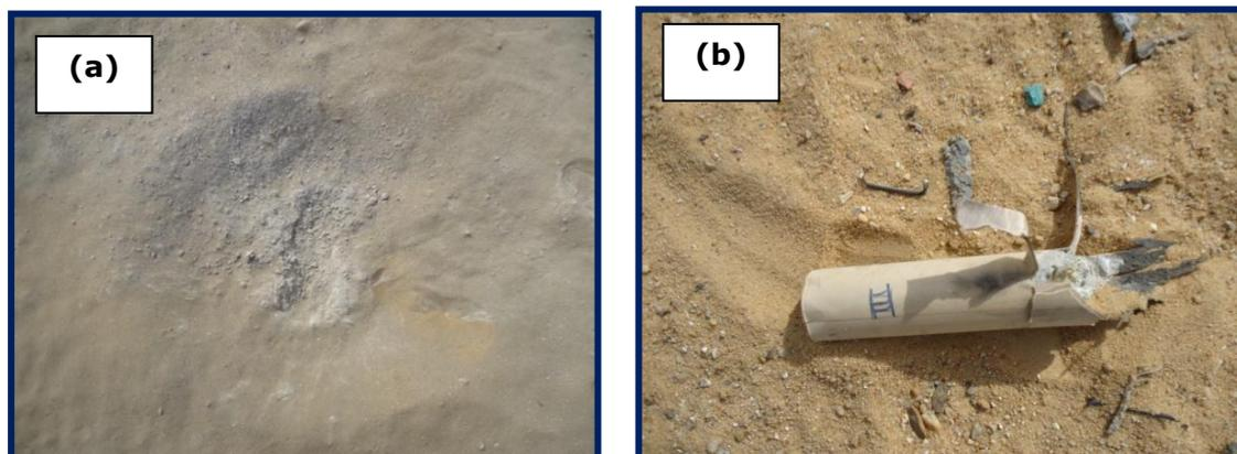
**Figure 14.** Ideal detonation for Al(100 nm)/TNT (a), no reaction for Al (10 μm) /TNT (b), at charge diameter of 40 mm.
