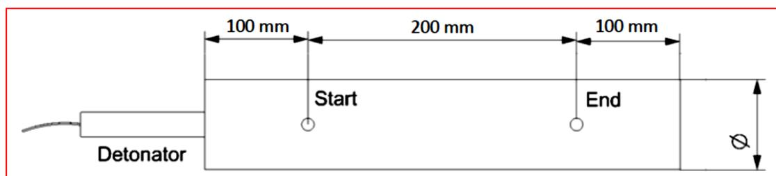
**Figure 8.** Detonation velocity measurement using an electronic timer
