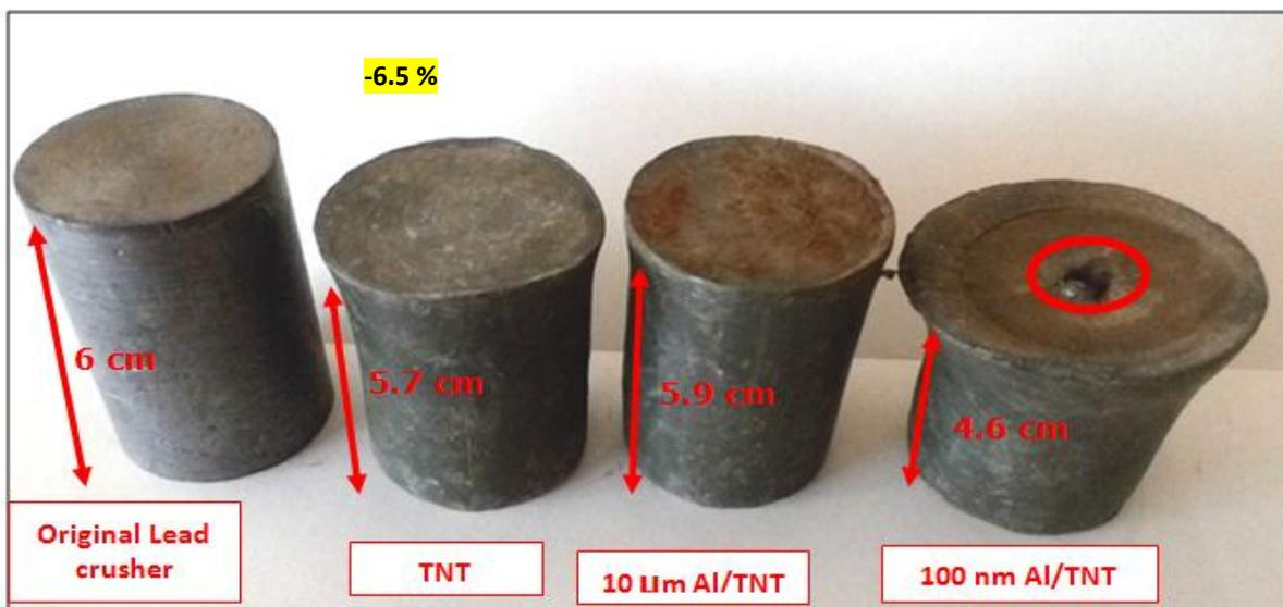
Figure 12. Effect of Al particle size on TNT brisance using Hess test
