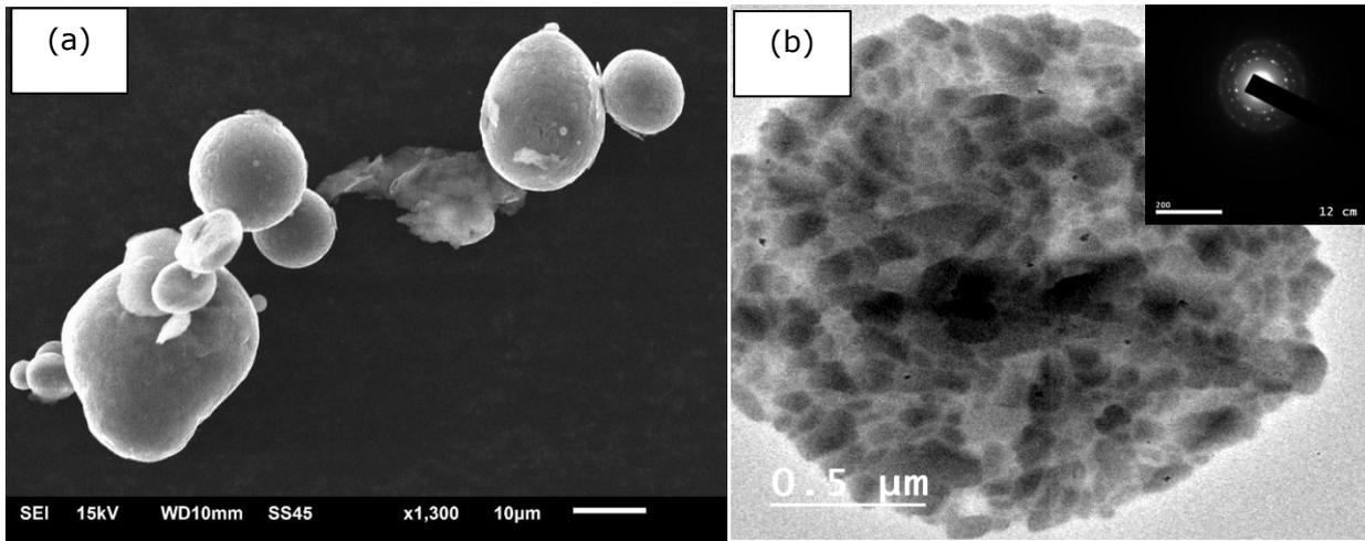
**Figure 9.** TEM micrograph of micron scale Al particles (a), nano-scale Al particles (b).
