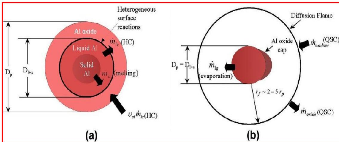
Figure 3. Sketch combustion model of aluminium particles.
