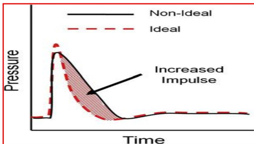
**Figure 2.** Pressure-time profile for an ideal vs. non-ideal detonation reaction.
