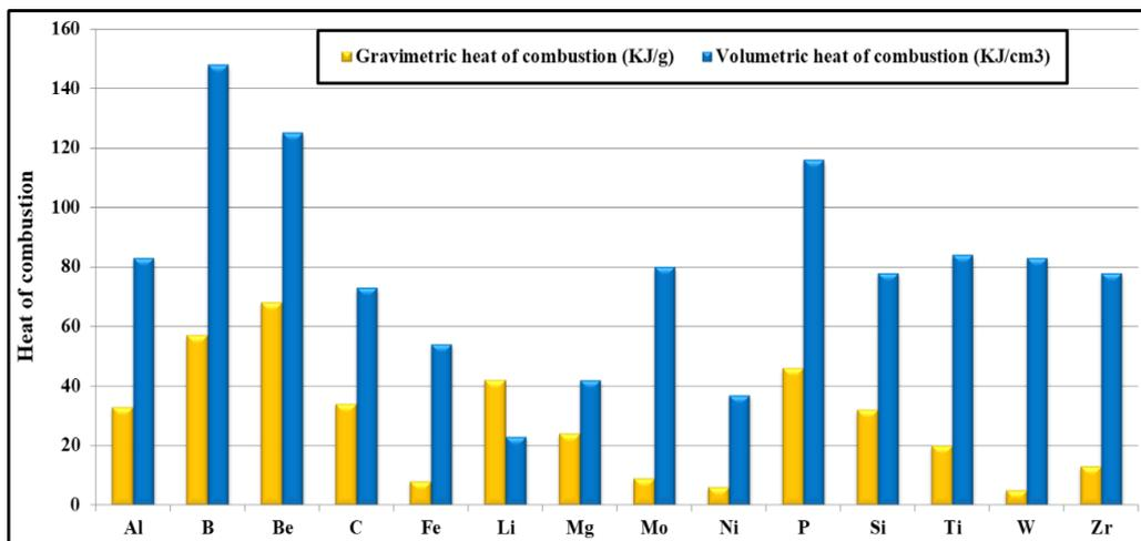
**Figure 1.** Heat output for common reactive fuels (Gravimetric and Volumetric).
