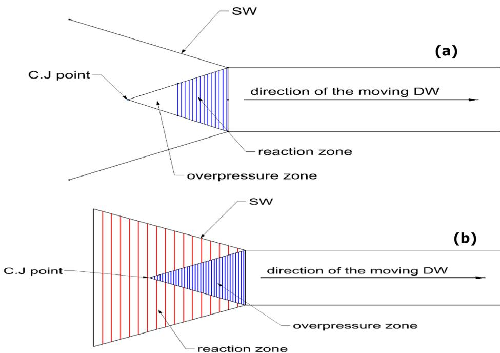
Figure 4. Schematic for ideal detonation reaction (a), and non-ideal detonation reaction (b).
