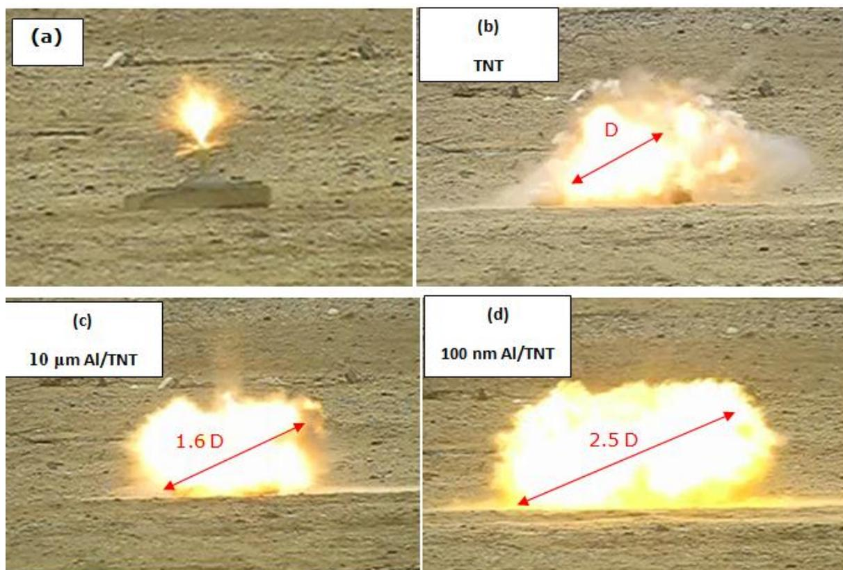
**Figure 13.** Hess test actions: moment of initiation (a), TNT (b), 10 $\mu\text{m}$  Al/TNT (C), 100 nm Al/TNT (d).
