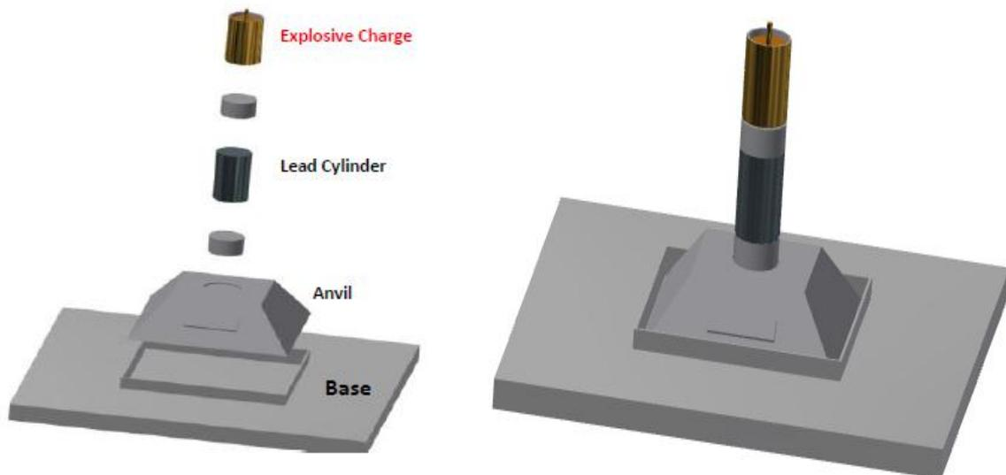
**Figure 7.** Setup for the determination of destructive effect by Hess test [9]
