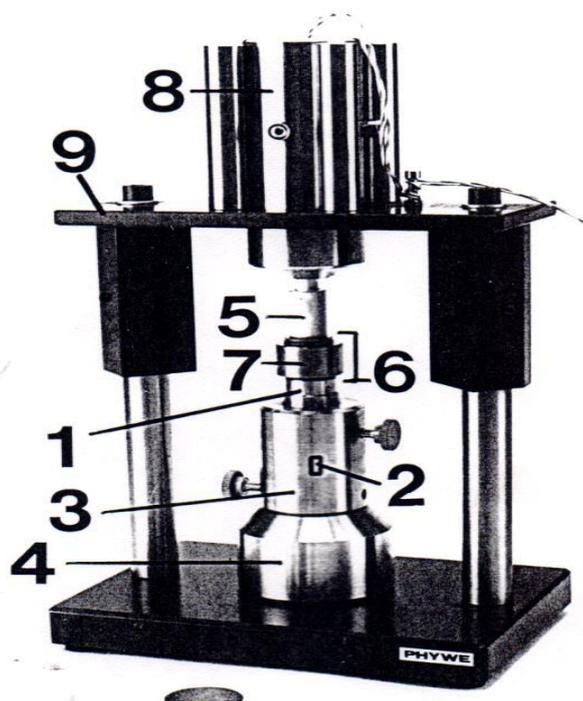
**Figure 6.** Schematic for destructive effect using Kast test [19].
