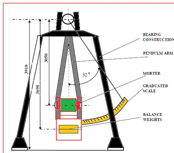
**Figure 5.** Schematic diagram of ballistic mortar [19]
