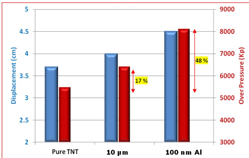
**Figure 10.** The impact of Al particle size on TNT workability
