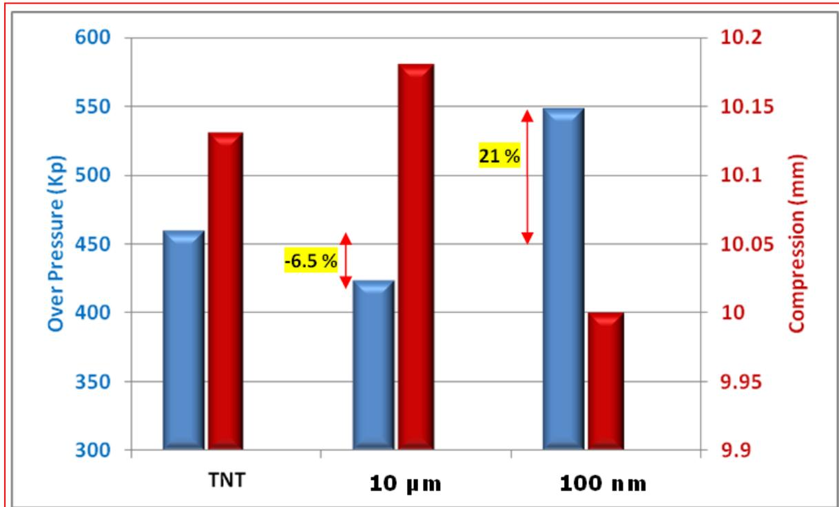
Figure 11. Impact of Al particle size on TNT brisance using Kast test.
