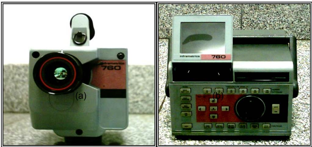
Figure (2.3) Inframetrics Infrared Radiometer model 760 IR Imaging Radiometer. (a) Inframetrics 760 thermal scanner. (b) Inframetrics thermal image-processing systems
