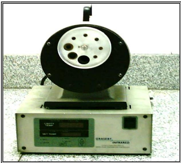
Figure (2.4) Graseby infrared black body IR radiator with temperature controlling unit
