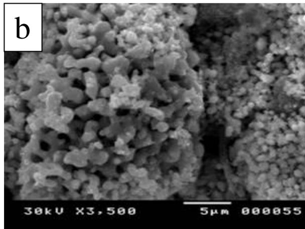
Fig. 3: SEM of CuFe<sub>2</sub>O<sub>4</sub>/ MgFe<sub>2</sub>O<sub>4</sub> core shell reduced at (a) 400 °C (b) 700 °C.
