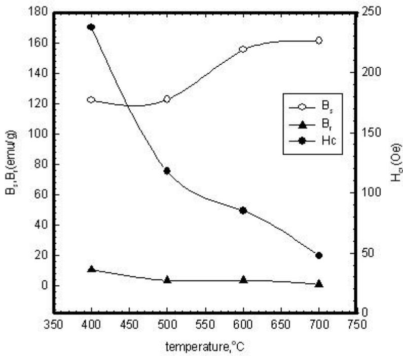
**Fig. 11: Relation between  $B_s, B_r, H_c$  and reduction temperature for  $CuFe_2O_4/MgFe_2O_4$  core/shell nanoparticles.**
