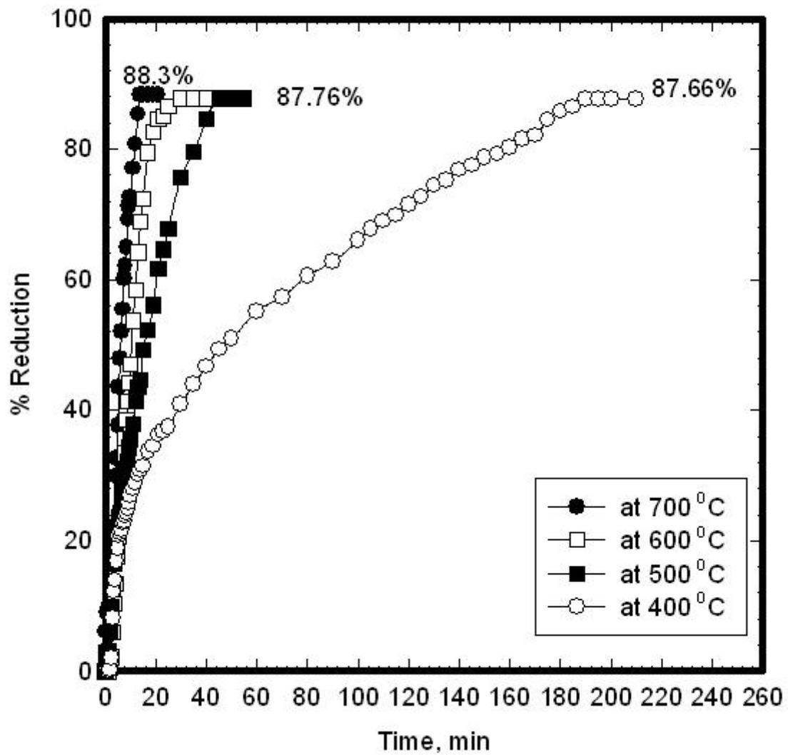
Fig. 6: Reduction curves of CuFe<sub>2</sub>O<sub>4</sub>/MgFe<sub>2</sub>O<sub>4</sub> core/shell at different temperature.
