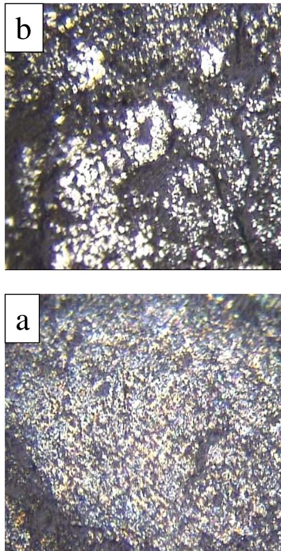
Fig. 5: Photomicrographs of reduced  $\text{CuFe}_2\text{O}_4/\text{MgFe}_2\text{O}_4$  core shell nanoparticles at different temperature (a) 500 oC (b) 700 oC (x400)
