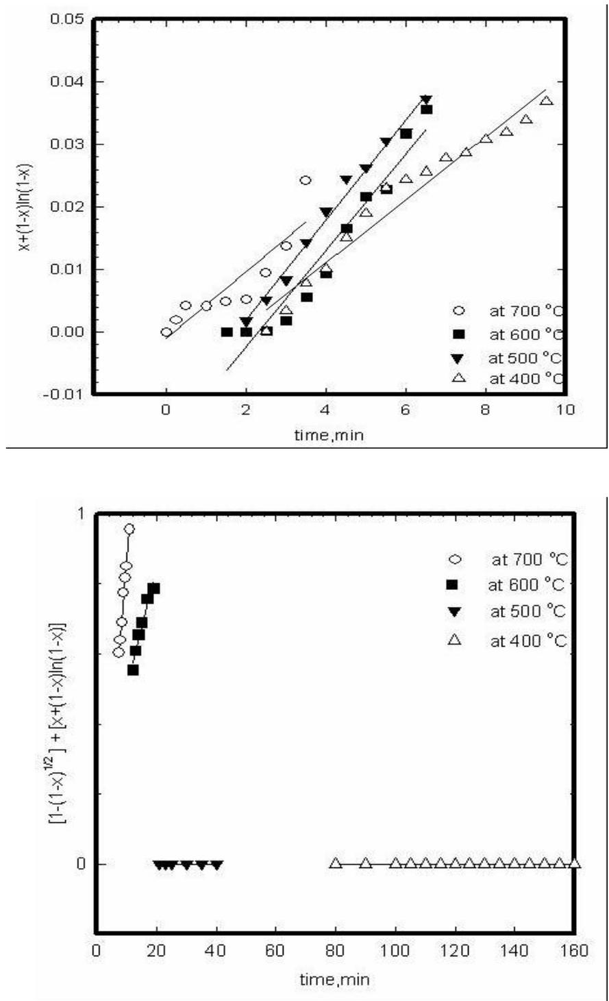
Fig. 9. (a) Application of gaseous diffusion control equation at the initial stages (b) Application of the combined chemical reaction and gaseous diffusion control equations at the final stages for CuFe<sub>2</sub>O<sub>4</sub>/MgFe<sub>2</sub>O<sub>4</sub>core/shell reduction at 400-700 oC .
