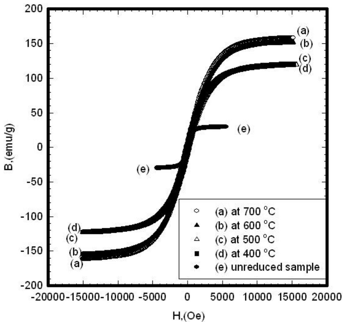
Fig. 10: B-H hysteresis loop of CuFe<sub>2</sub>O<sub>4</sub>/MgFe<sub>2</sub>O<sub>4</sub> core/shell reduced at different temperature.
