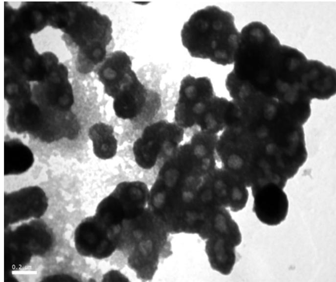
Fig. 1:TEM of CuFe<sub>2</sub>O<sub>4</sub>/MgFe<sub>2</sub>O<sub>4</sub>core/shell nanoparticles.
