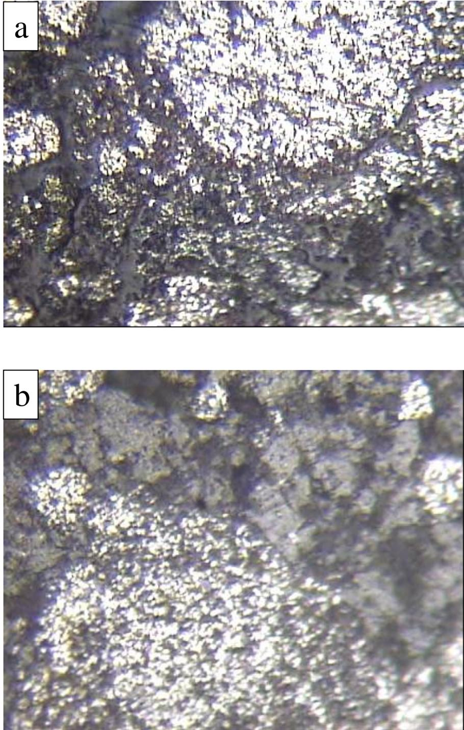
Fig. 8 : Photomicrograph of CuFe<sub>2</sub>O<sub>4</sub>/MgFe<sub>2</sub>O<sub>4</sub> core/shell sample partially reduced at 600 oC to(a) 80% (b)30% ( x 400).
