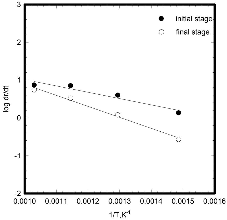
Fig. 7. Arrhenius plots for CuFe<sub>2</sub>O<sub>4</sub>/MgFe<sub>2</sub>O<sub>4</sub> core/shell reduction at the initial and final stages.
