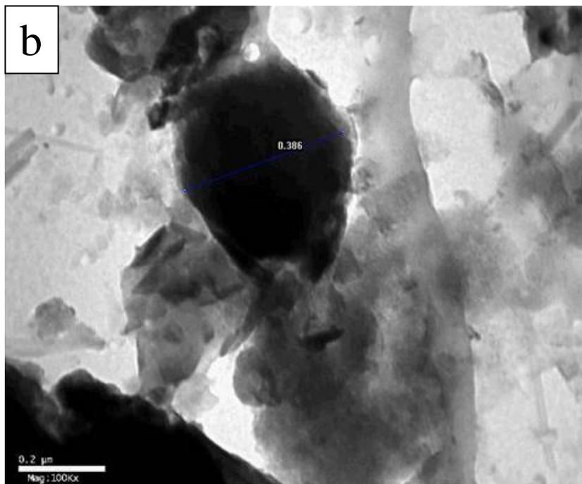
Fig. 4: TEM photos of (a) unreacted  $\text{CuFe}_2\text{O}_4/\text{MgFe}_2\text{O}_4$  core shell nanoparticles (x 120K), (b) reduced  $\text{CuFe}_2\text{O}_4/\text{MgFe}_2\text{O}_4$  core shell nanoparticles at 700 oC (x 100K).
