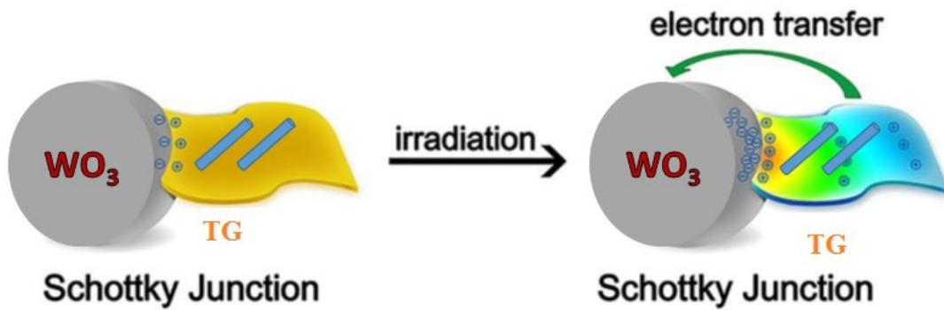
Figure (12) An illustration of the Schottky junction between TG/WO<sub>3</sub>.
