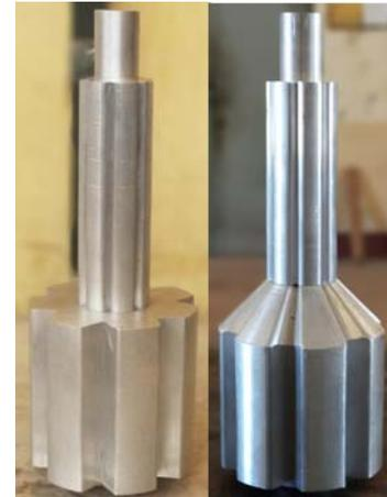
**Figure 23.** Taper and sharp mandrels used in SPRM.
