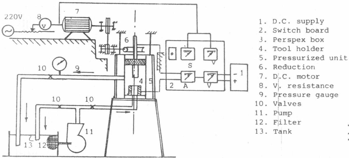
Fig. (3): Schematic layout of ECM set-up.
