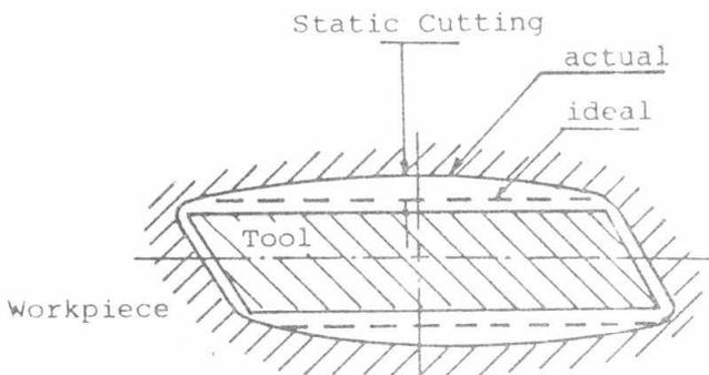
Fig. (1): Effect of Static Cutting on final Shape (4).
