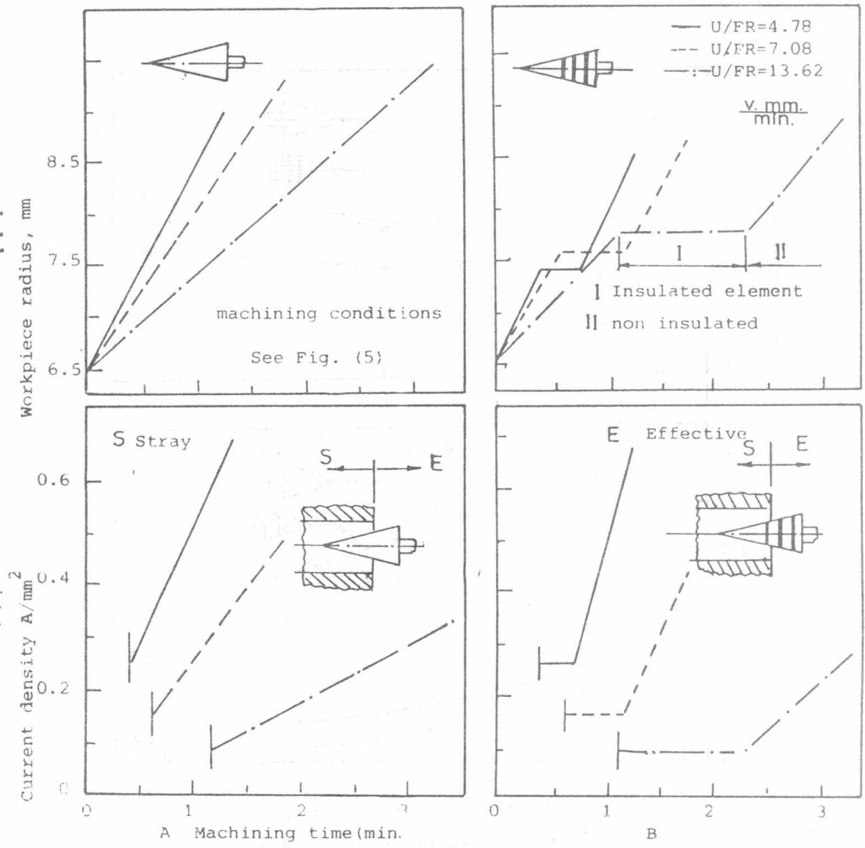
Fig. (8): Effect of machining time on process variables.
