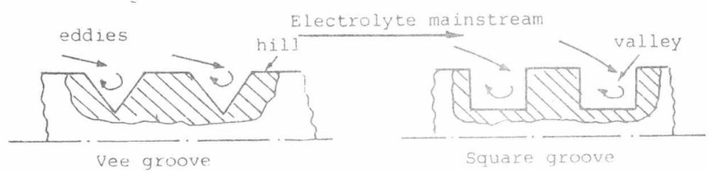
Fig. (7): Analysis of flow mainstream over recessed cathode.
