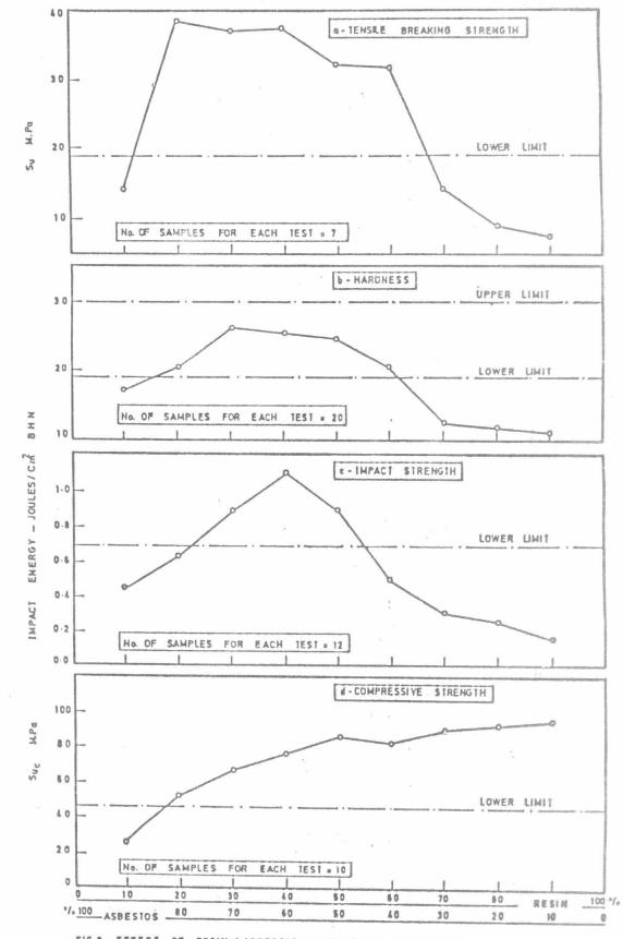
FIG.2 - EFFECT OF RESIN / ASBESTOS CONTENT ON MECHANICAL PROPERTIES OF
