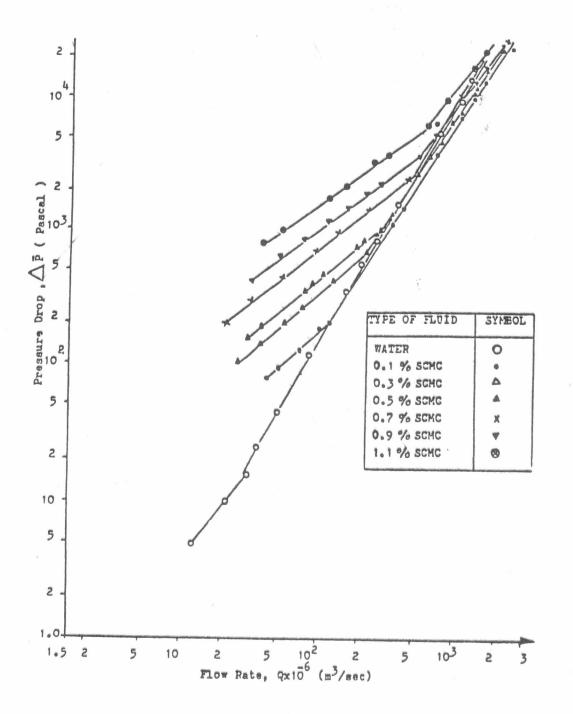
Fig.(2), Pressure drop in 17.5 mm smooth pipe.
