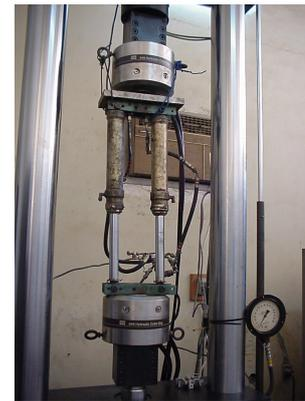
Fig. 6 Hydraulic cylinders clamped between the two grips of the MTS machine
