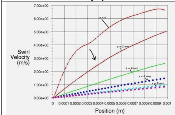
Fig. 5. Plasma swirl velocity at a distance z [mm] downstream torch shield along the radius of the jet with secondary gas swirl coherent with the primary gas swirl. Picture taken from [22].
