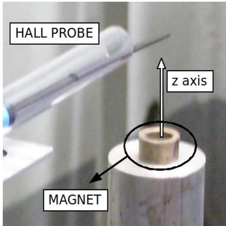
Fig. 7. Experimental setup for 2-D reconstruction with Hall effect probe of magnetic flux generated by the permanent magnet embedded in the Komatsu torch (internal diameter: 10mm; external diameter: 14.8mm; height: 8mm) as from patent [12]. Picture taken from [22].
