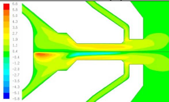
Fig. 9. Comparison of plasma swirl velocity [m/s] from simulation for the Komatsu plasma torch with (below) and without (above) magnetization apparatus under the following operating conditions: 120A, plasma gas pressure (air)=3 bar; secondary gas pressure (air)=1 bar; nozzle diameter=1.37mm. Picture taken from [22].
