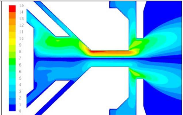
Fig. 2. Plasma swirl velocity [m/s] from simulation for the vented (upper-half) and non-vented case (lower-half). Picture taken from [22].
