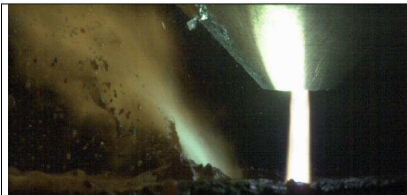
Figure 11. Piercing of a 40 mm MS slab using non perfectly aligned torch head components (1.9 mm nozzle, 250 A, cut plasma/shield gas: O<sub>2</sub>/air, 1,000 fps, 1/20,000 shutter time). Pictures taken from [20].
