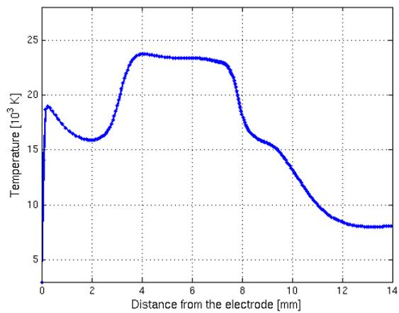
Fig. 10. Plasma temperature [K] on the axis of the torch from simulation for the Komatsu plasma torch with magnetization apparatus under operating conditions as in Fig. 9. Picture taken from [22].
