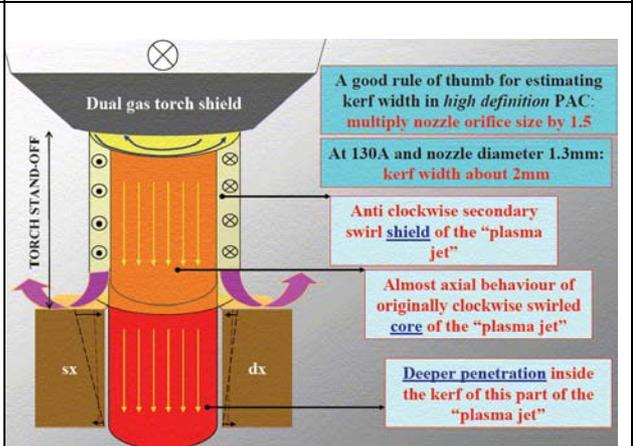
Fig. 4. Qualitative explanation of formation of bevel angle based on evidence of the effects of anticlockwise secondary swirl. Picture taken from [22].
