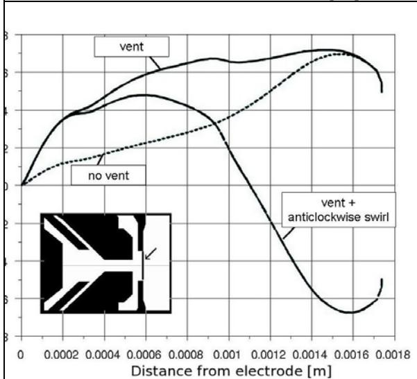
Fig. 3. Radial behavior of plasma swirl velocity [m/s] at the nozzle exit from simulation for the vented case with two types of secondary gas swirl and for the non-vented case. Picture taken from [22].
