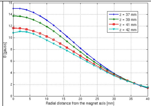
Fig. 8. Magnetic field magnitude [gauss] of the Komatsu magnet as function of radial distance from the axis [mm] and for different distances from the magnet [mm] (cathode tip at z = 37 mm and nozzle exit at z = 42 mm). Picture taken from [22].
