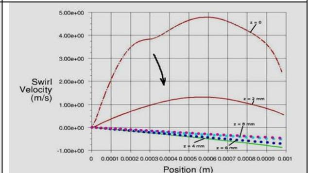
Fig. 6. Plasma swirl velocity at a distance z [mm] downstream torch shield along the radius of the jet with anticlockwise swirl of the secondary gas. Picture taken from [22].
