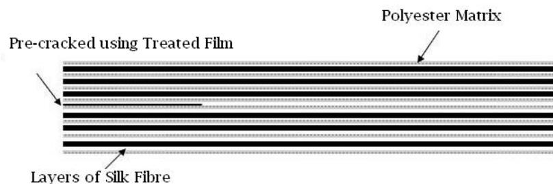
Fig. 1. Cross-section of the laminated silk fiber/polyester composites
