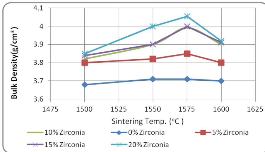
**Figure (2):** Bulk density of ceramic composites, fired at different firing temperatures.
