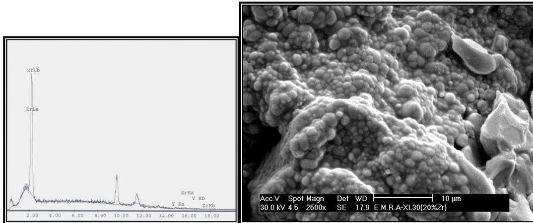
**Figure (8):** EDX of clusters of fine-grained ZrO<sub>2</sub> particles
