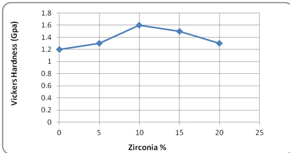
**Figure (10):** Effect of weight percent of Zirconia on vickers hardness of the ceramic composite.
