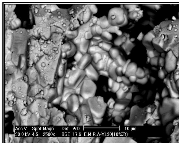
**Figure (7):** The pinning effect of ZrO<sub>2</sub> on the grain growth of Al<sub>2</sub>O<sub>3</sub>
