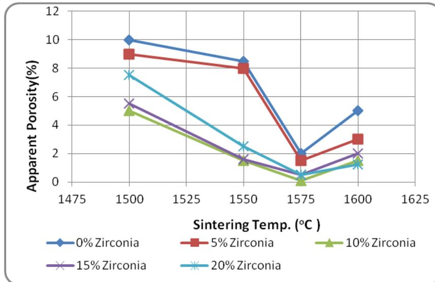
**Figure (3):** Apparent porosity of ceramic composites fired at different firing temperatures.
