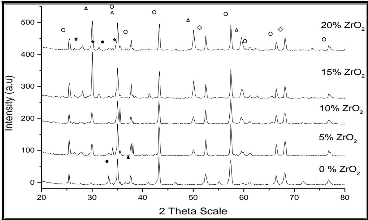
**Figure (4):** XRD patterns of the tested composite specimens, where  $\circ$  : Corundum,  $\Delta$  t-ZrO<sub>2</sub>,  $\star$  m-ZrO<sub>2</sub>,  $\bullet$  SiC and  $\blacktriangle$  SiC-2H
