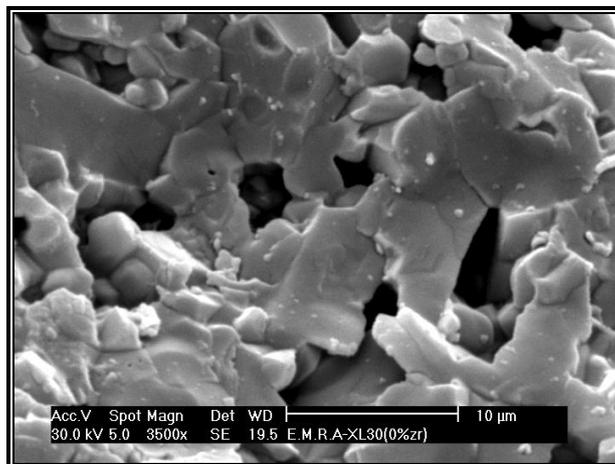
**Figure (6):** SEM of Alumina grain growth
