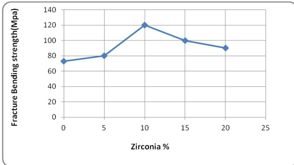
**Figure (9):** Effect of weight percent of Zirconia on flexural bending strength of the ceramic composite.
