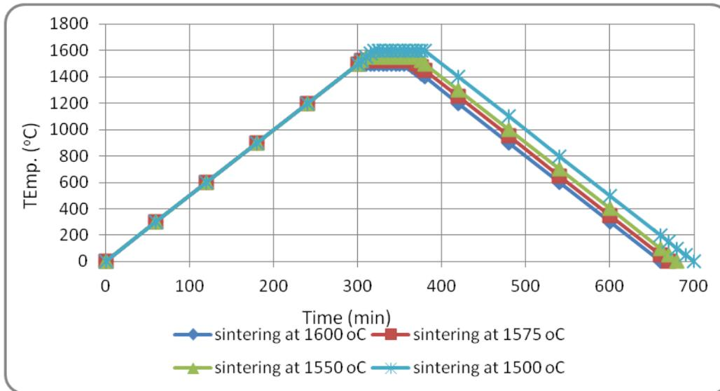
**Figure (1):** Sintering cycles of different ceramic composites batches.
